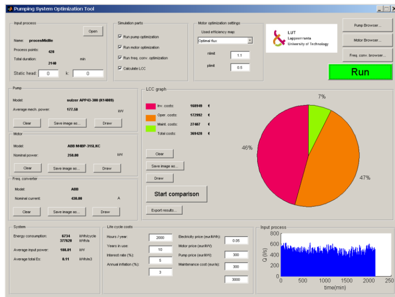
Fig. 1. Pumping System Optimization Tool's main window.
