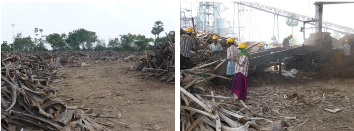
Figure 11. Biomass store yard (left) and crushing unit (right) at power plant. (Photos Arvo Leinonen)
