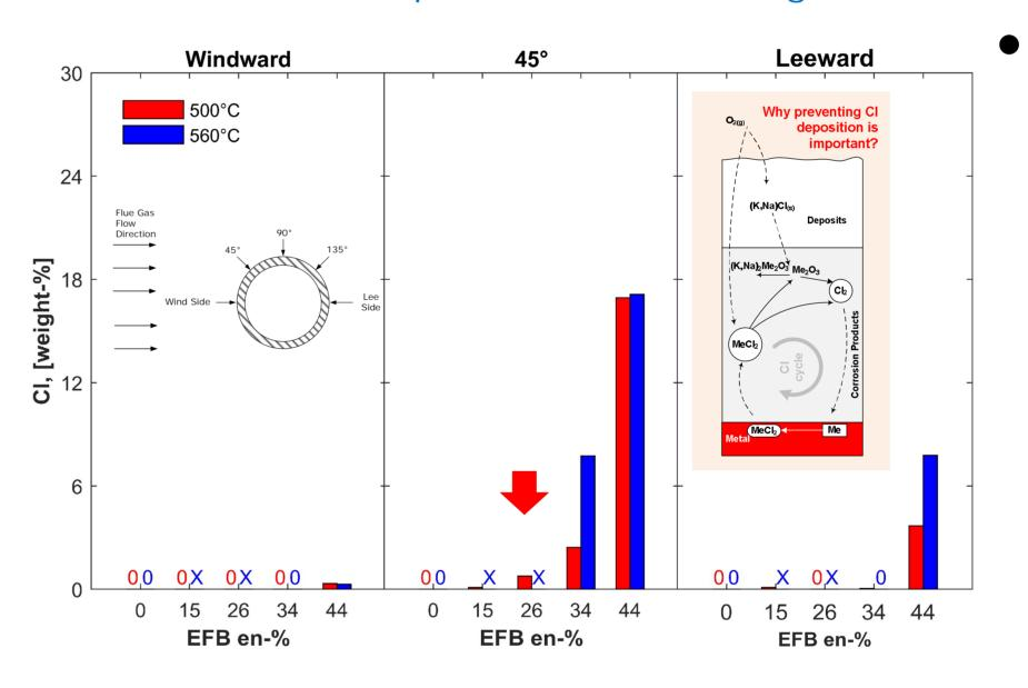
Depending on superheater design, material temperature and grade the risk of corrosion may start in the range of 25 en-% to 35 en-% EFB.
