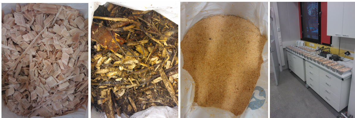
Figure 1. Wood chip, forest chip and sawdust samples, and the wood chip sample after splitting into smaller partial samples.
