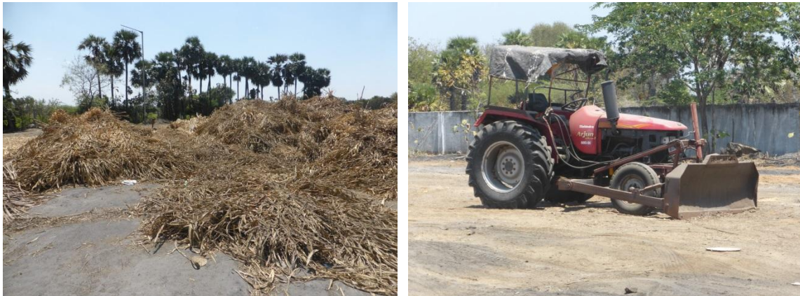
Figure 52. Drying of energy grass (left) and tractor with front end loader for spreading and collecting of biomass on the drying field (right).
