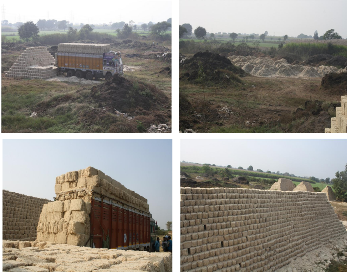
Figure 61. Bagasse lorry load (up and right), biomass storage yard (up and left), unloading of bagasse bales from lorry at storage yard (down and left) and bagasse bales piles (down and right).
