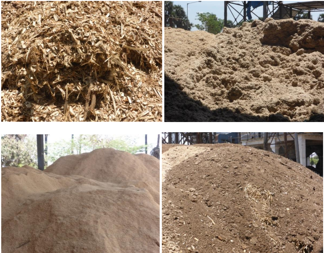
Figure 49. Some biomass fuels used at the power plant; Prosopis juliflora (up and left), bagasse (up and right), rice husk (down and left) and chicken litter (down and right).
