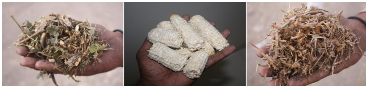
Figure 63. Different biomass fuels used at the power plant. Cotton stalks (left), maize cobs (middle) and soybean husk (right).
