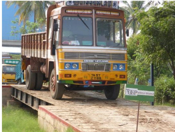
Figure 43. Biomass payload is weighed at the gate using lorry scales (Photo by Arvo Leinonen).
