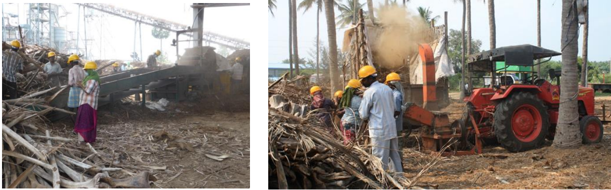
Figure 46. Coconut frond comminution with stationary crusher (left) at biomass yard and mobile chipper (right) outside the power plant area (Photos by Arvo Leinonen and Karthikeyan Natarajan).
