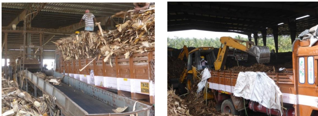
Figure 44. Manual unloading of plywood biomass directly to the crusher (left) and unloading of sawmill residues by excavator (right) (Photos by Arvo Leinonen and Karthikeyan Natarajan).
