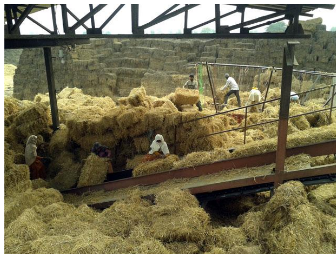
Figure 67. Loading of straw bales to the conveyor transferring material to the crusher at the Universal Power plant in Channu Village (Dailypost 2014).
