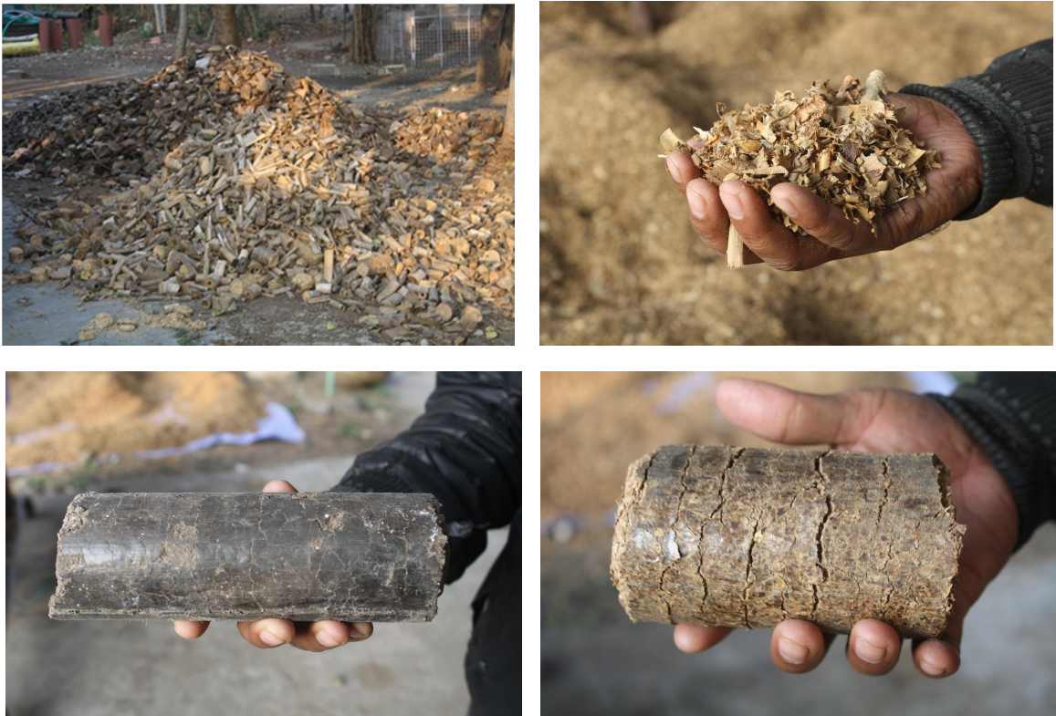
Figure 60. Different biomass fuels used at power plant. Chipped bamboo (up and left), shavings (up and right), bagasse briquettes (down and left) and soybean briquettes (down and right) (Photos by Karthikeyan Natarajan).
