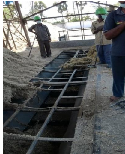
Figure 54. Biomass feeding conveyor (up and left) for Prosopis juliflora chips and rice husk to the boiler, biomass feeding conveyor for sugar cane trash and grass chops (up and right) at power plant, feeding (grass chops etc.) to the conveyor (down and left) and feeding grate at the at the beginning of biomass conveyor (down and right).
