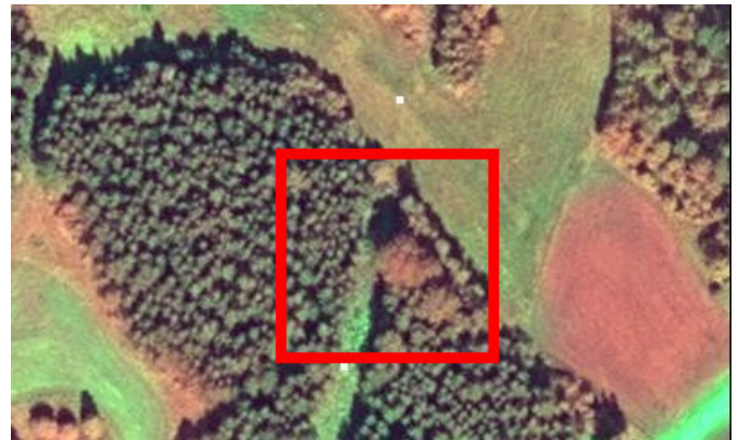
Fig. 1: Risk detection example, 0.5 m resolution, false color. The image shows a 20 kV power line segment, whose end-points are marked with white markers. The red square points a location in which the width of the power line corridor is less than the specified limit, 7.5 m.
