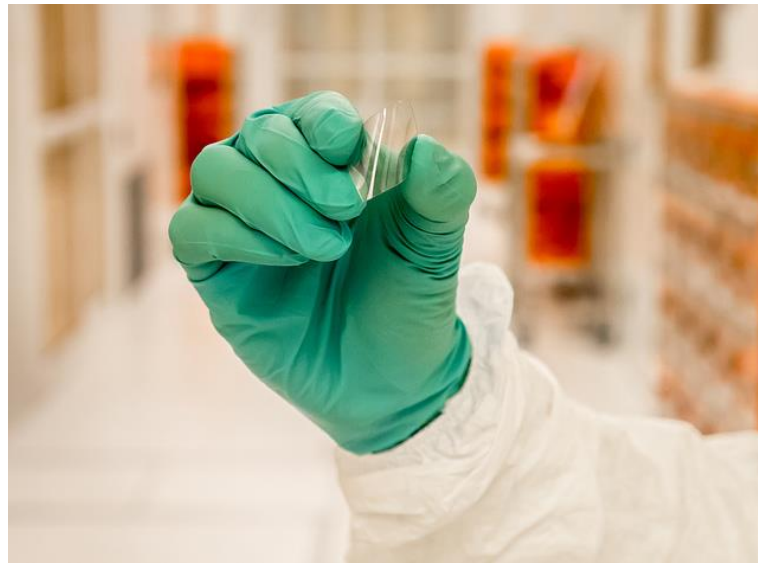
Figure 13. An array of flexible, transparent TFTs developed at Argonne National Laboratory. (Mark Lopez/Argonne National Laboratory)
