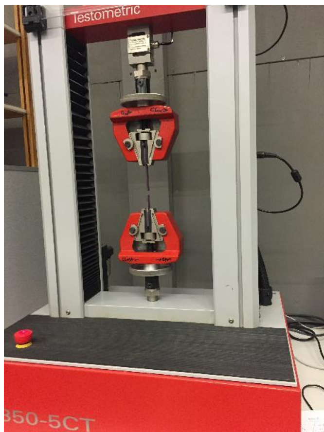
Figure 23 Dog-bone being tested with testometric tensile testing machine (Arcada plastic laboratory, June 2014)
