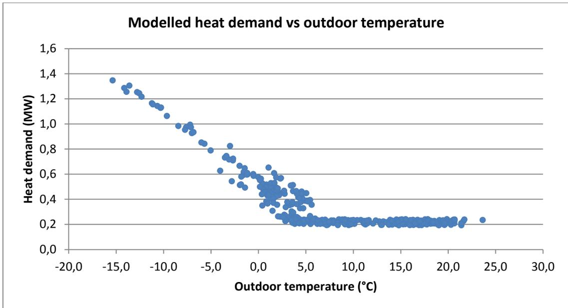
Figure 5-7. Modelled heat demand as a function of outdoor temperature for the Honkasuo residential area
