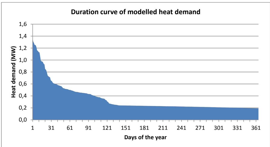
Figure 5-8. Duration curve of the modelled heat demand in Honkasuo
