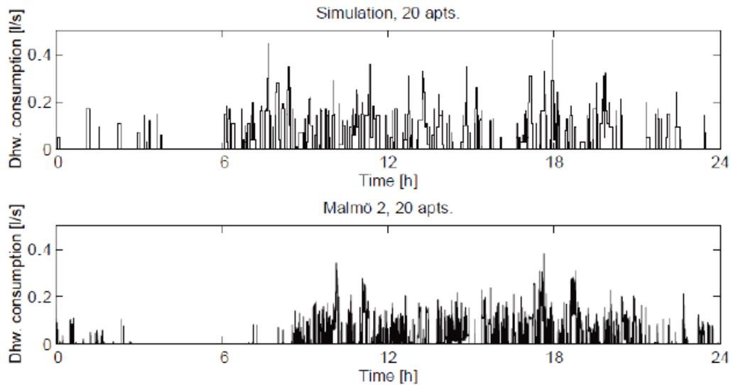
Figure 4-5. Comparison of simulated and measured hot water consumption values [10]
