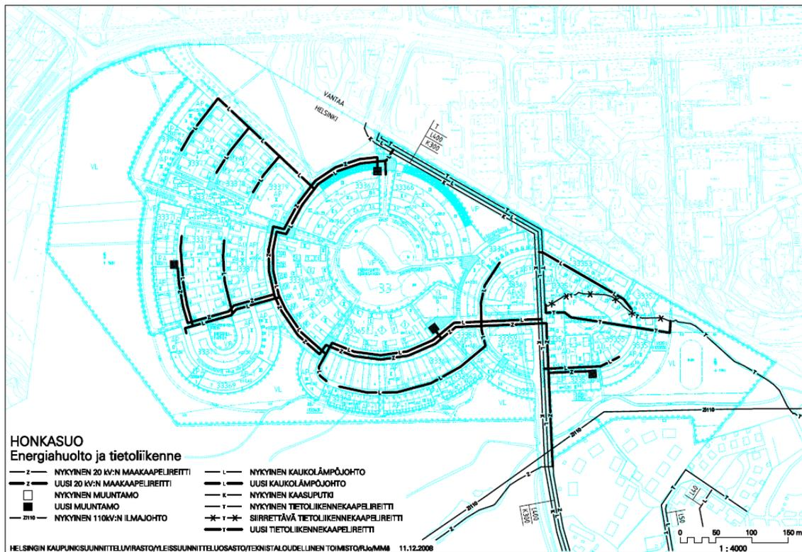
Figure 5-3. The district heating network planned for Honkasuo with heating pipes marked by "L-" [24]
