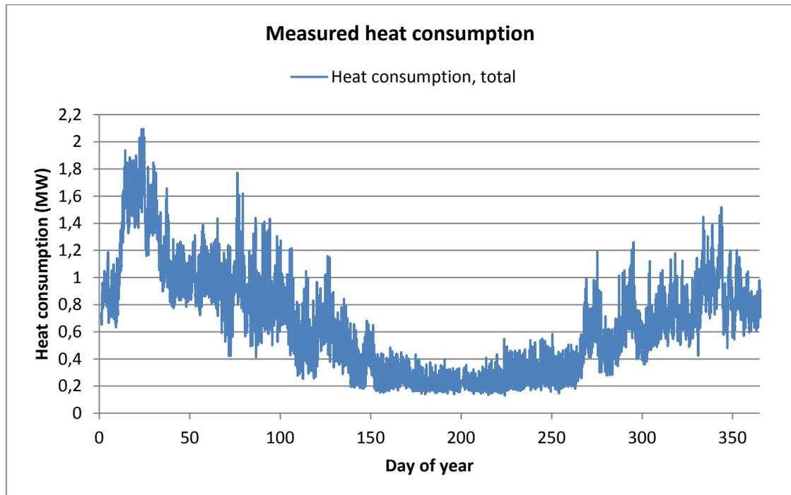
Figure 5-9. Measured heat consumption scaled to the same housing area as in Honkasuo
