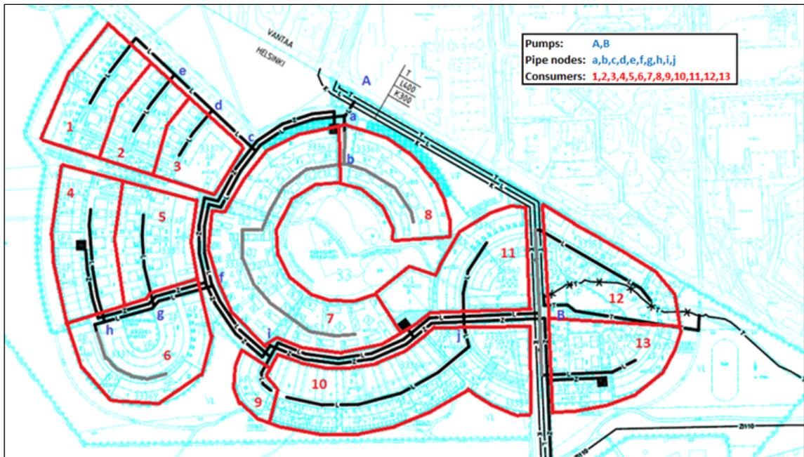
Figure 5-15. Simplified model of the heat distribution in Honkasuo
