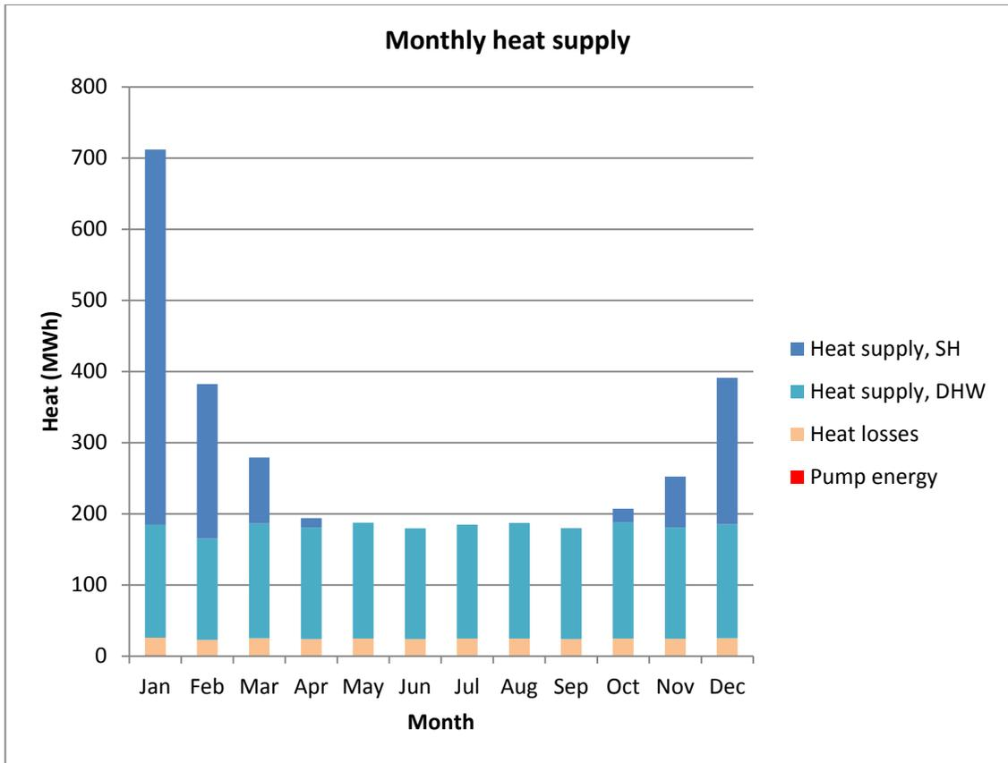
Figure 5-16. Simulated heat supply and energy losses in Honkasuo
