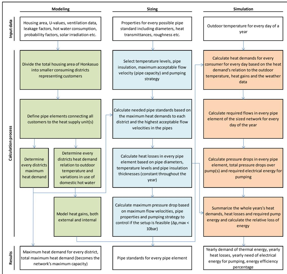
Figure 5-4. Simulation program structure
