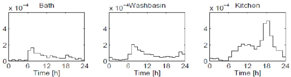
Figure 4-2. Probabilities of a hot water tap occurring at a given time [10]
