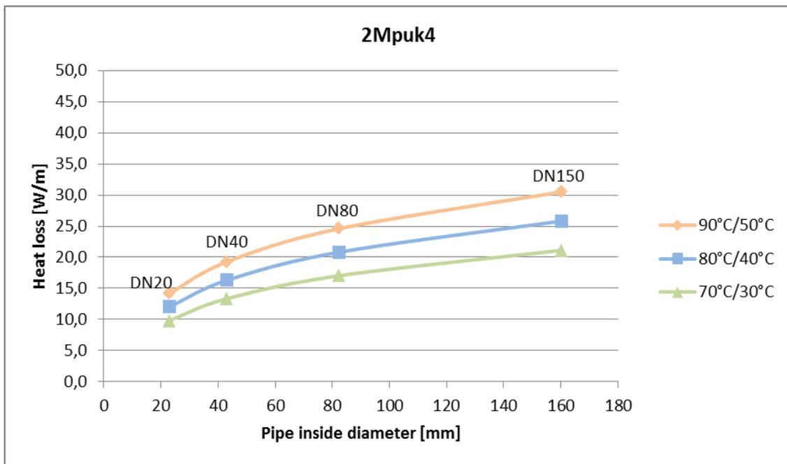
Figure B-4. Heat loss in single pipes of insulation class 4
