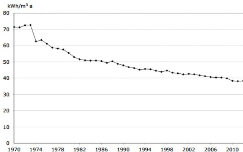
Figure 2-3. Specific heat consumption in district heated buildings in Finland [7]
