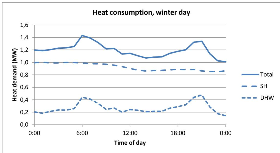
Figure 5-13. Determined heat consumption in Honkasuo during a winter day
