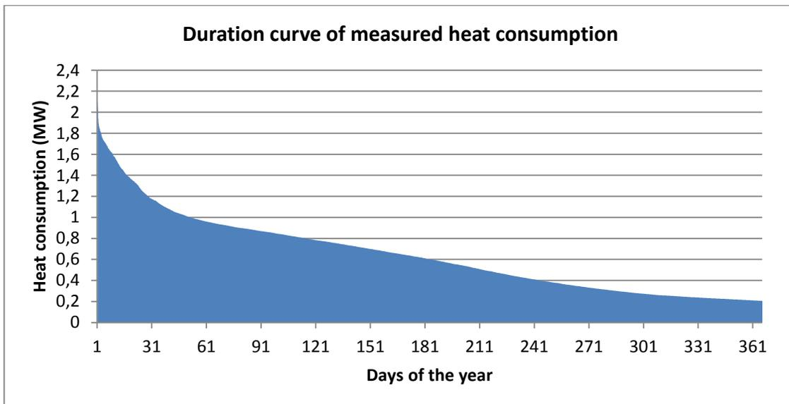
Figure 5-11. Duration curve of the measured heat consumption scaled to the same housing area as in Honkasuo
