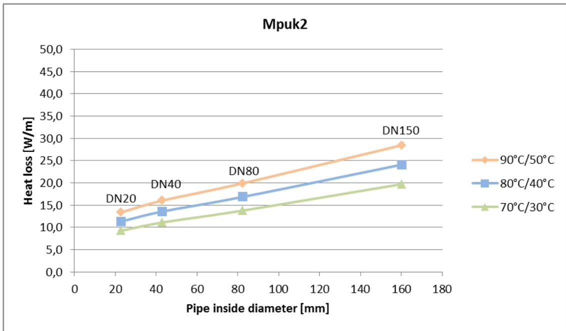
Figure B-6. Heat loss in twin pipes of insulation class 2
