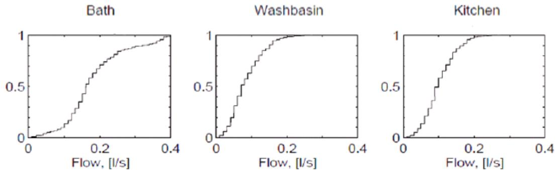
Figure 4-3. Probabilities of a specific volume flow of hot water [10]
