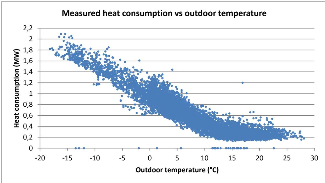
Figure 5-10. Measured heat consumption, scaled to the same housing area as in Honkasuo, as a function of outdoor temperature
