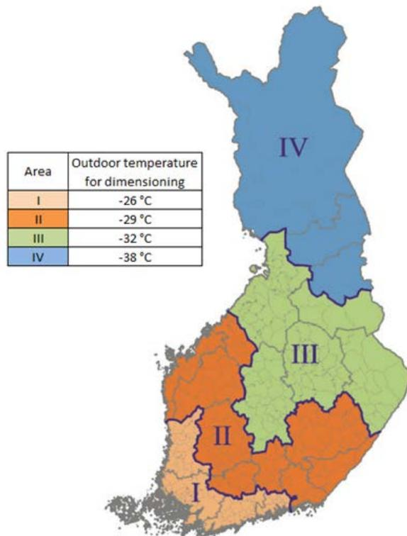
Figure 4-1. Dimensioning outdoor temperatures used in Finland [14]
