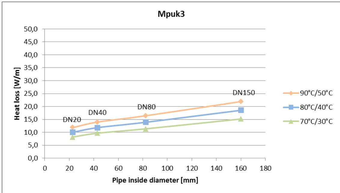
Figure B-7. Heat loss in twin pipes of insulation class 3
