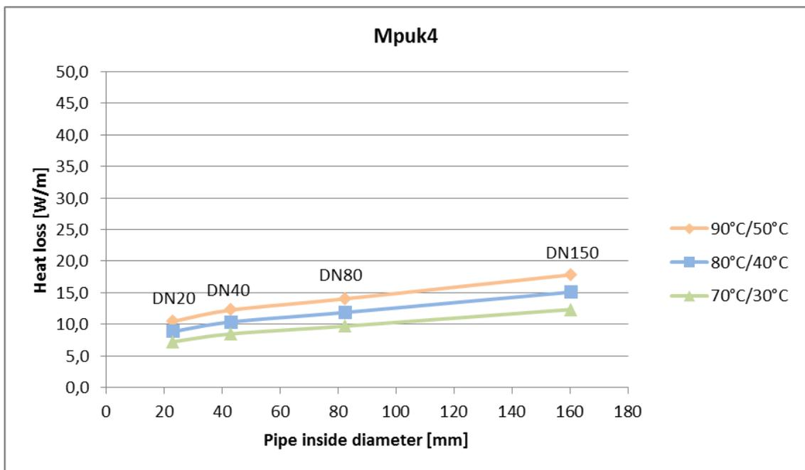
Figure B-8. Heat loss in twin pipes of insulation class 4
