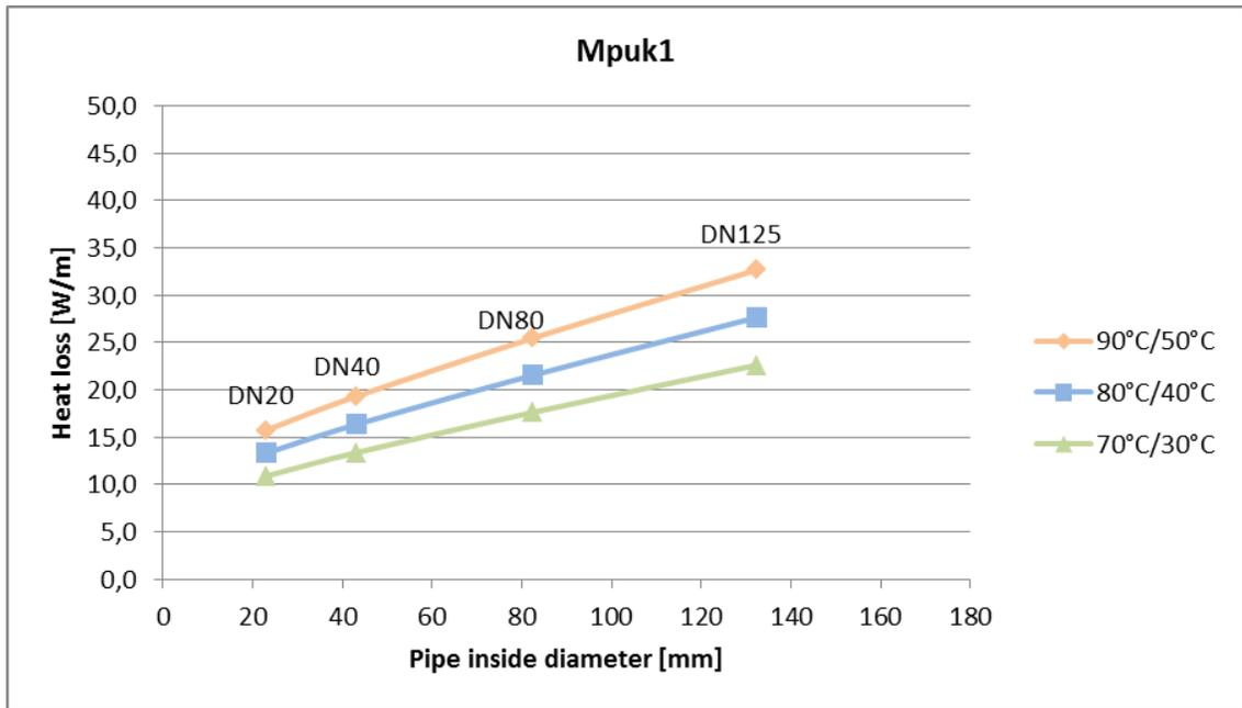
Figure B-5. Heat loss in twin pipes of insulation class 1
