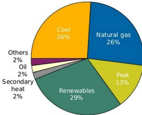
Figure 2-2. Fuel consumption in production of district heat and CHP 2013 [8]
