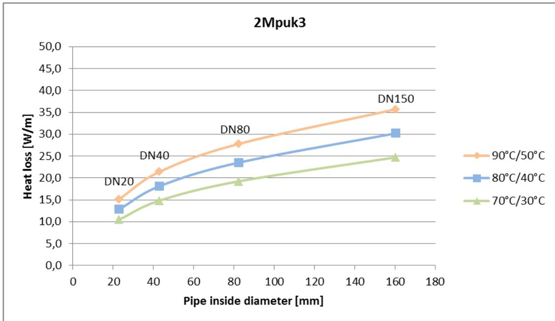
Figure B-3. Heat loss in single pipes of insulation class 3
