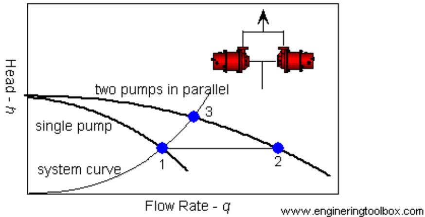
Figure 4-7. Characteristics for a single pump and two pumps in parallel [22]
