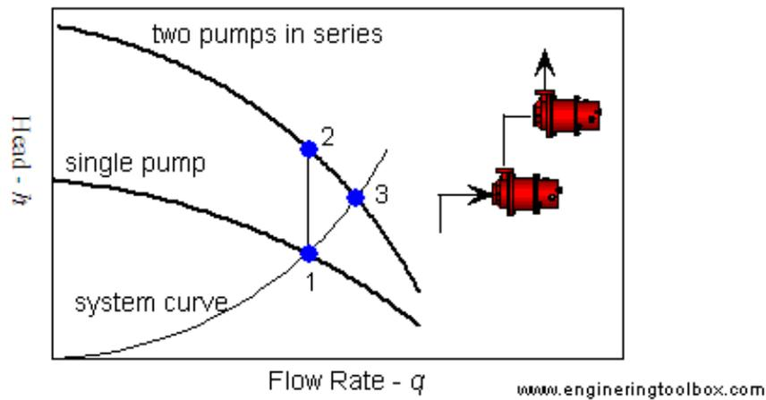
Figure 4-8. Characteristics for a single pump and two pumps in series [22]
