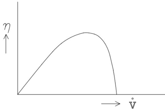
Figure 4-9. Efficiency characteristics of a centrifugal pump [21]
