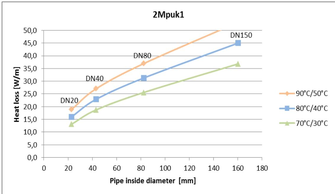
Figure B-1. Heat loss in single pipes of insulation class 1
