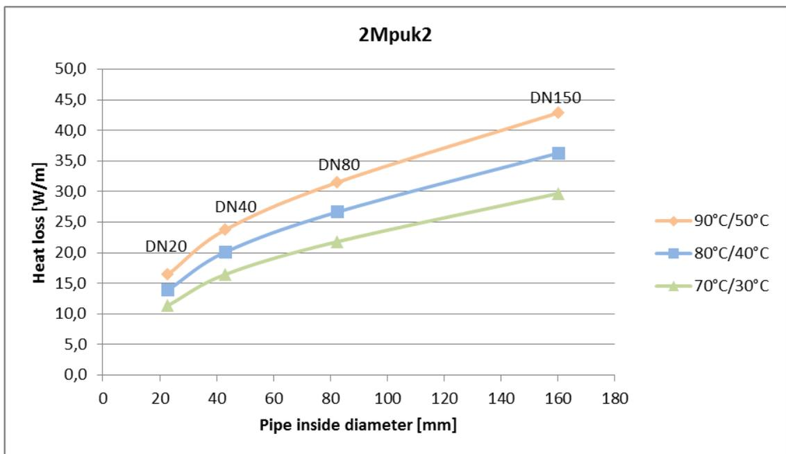
Figure B-2. Heat loss in single pipes of insulation class 2
