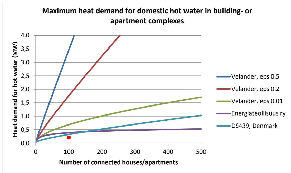
Figure 5-14. Maximum heating demand for domestic hot water in connected houses or apartments according to different formulas [1]
