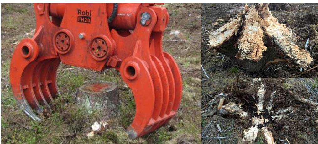
Figure 16. Soil disturbance and foreign matter can be minimized leaving roots in place.
