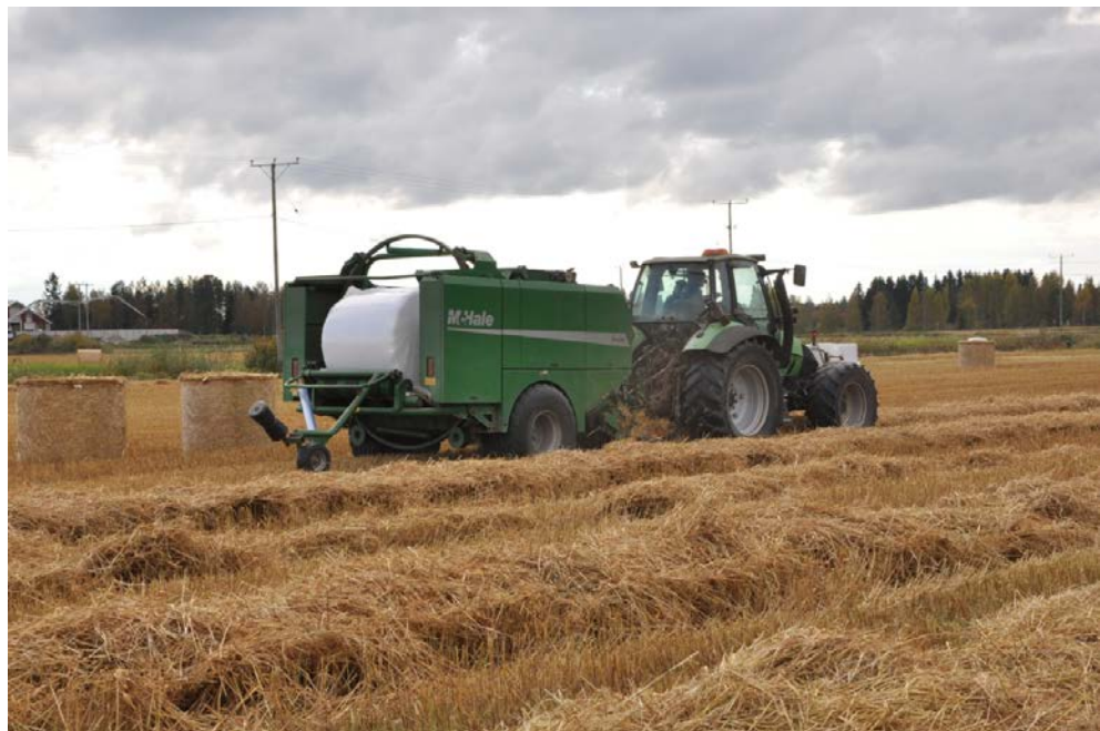
Figure 1. The round bales were made with an integrated round baler wrapper either without wrapping or wrapped with a plastic film.
