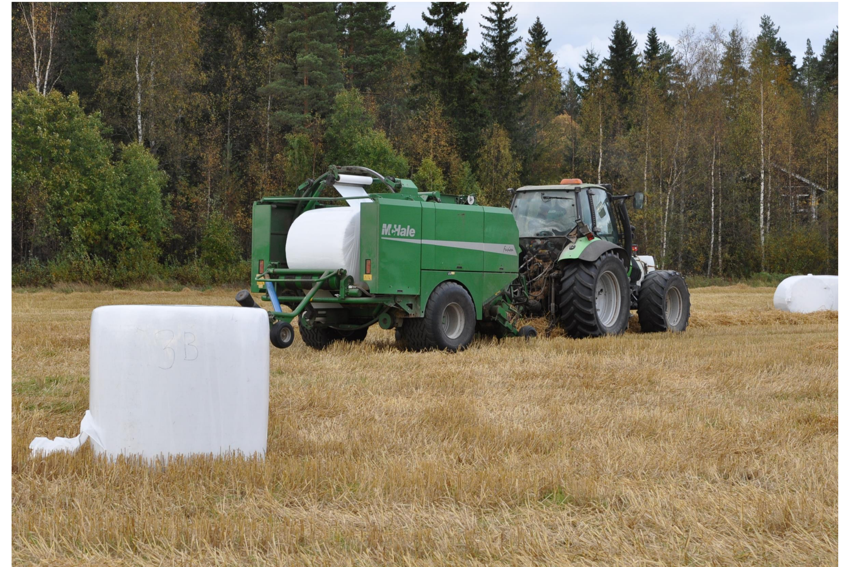
Figure 1. The barley straw was baled with an integrated round baler wrapper with full bale density setting.
