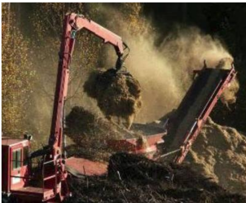
Figure 6.3. Crushing reed canary grass bales (Ajanko-Laurikko 2009) Photo: VTT
