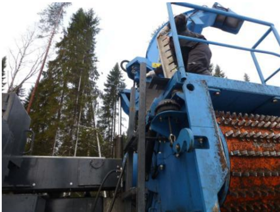
Figure 3.2. Maintenance of a chipper (here changing the blades of the cutting drum) is one of the riskiest tasks in terms of accidents. In many cases, the work is done above ground level, and sharp parts of the machine have to be handled. (Photo: Kari Ojanen, FIOH)
