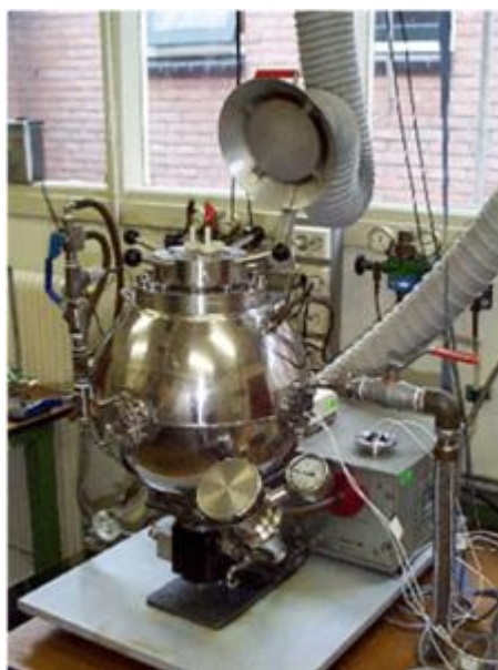
Figure 5.1. A 20-litre sphere used for dust explosion measurements (Wilén et al. 2013, Wilén et al. 1999) Photo: TNO
