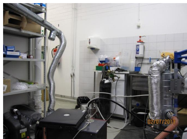
Figure 1b. Sample line for measuring tracer particles "blown" from the filter.
