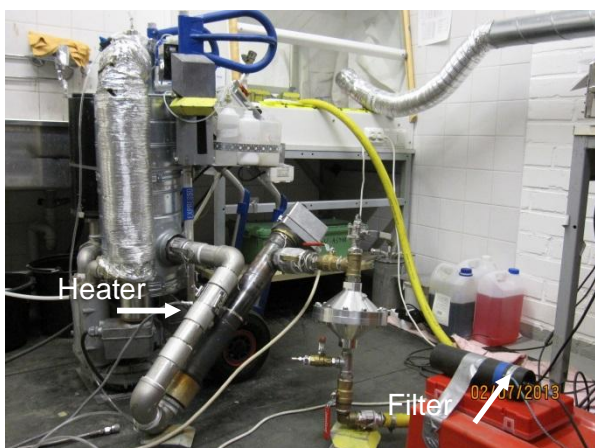
Figure 1a Measurement set-up for filter collection experiments with active tracer particles.
