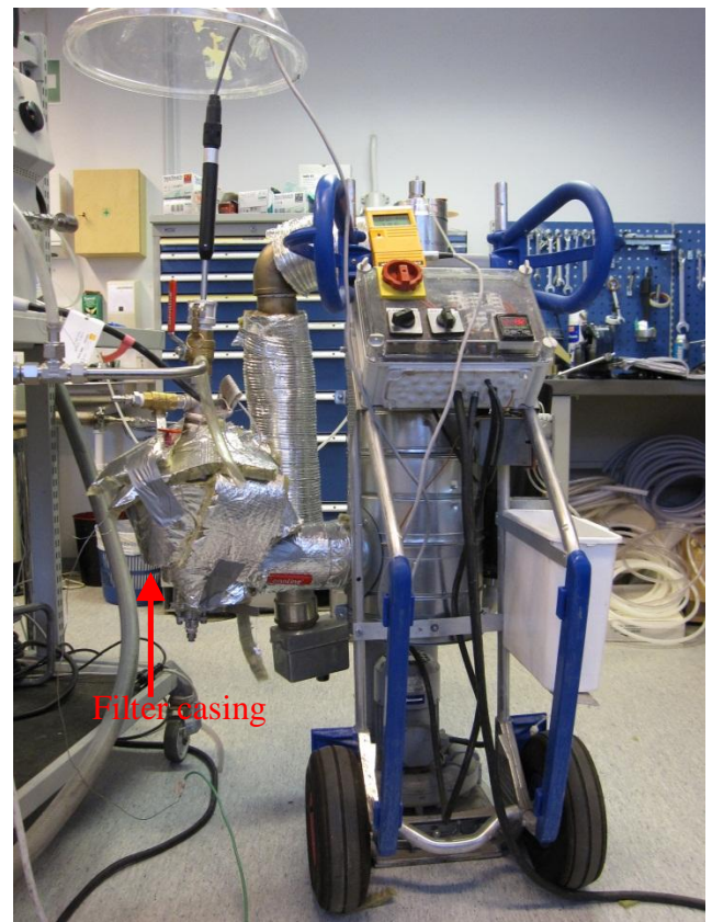
Fig. 1c. Measurements set-up for filter collection of the produced particles (09/2011).
