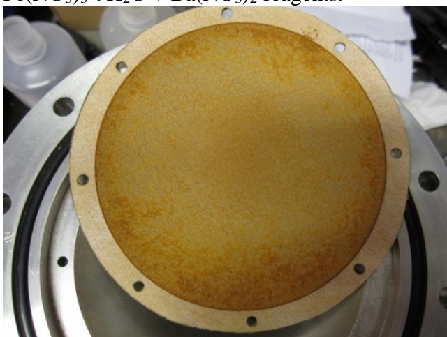
Fig. 22c. The collecting side of the filter after the experiment on 31.8.2011 used for collecting particles produced from \text{Fe}(\text{NO}_3)_3 \cdot 9\text{H}_2\text{O} and \text{Fe}(\text{NO}_3)_3 \cdot 9\text{H}_2\text{O} + \text{Ba}(\text{NO}_3)_2 reagents.
