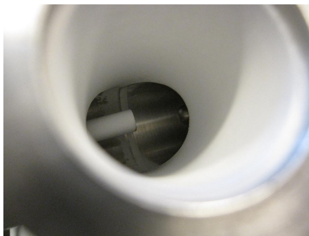
Fig. 3b. The impaction plate installed in the flow channel of the experimental set-up. The nose of the plate ("bullet") is seen on the right, and the tube where the produced particles are "blown" from the cyclone to experimental set-up on the left.
