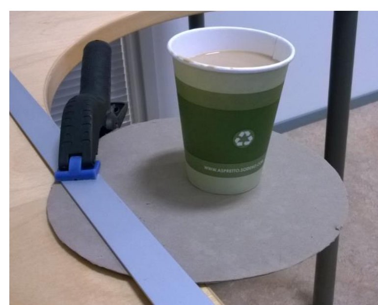
Right: Laboratory hand made sheet from fiber waste sludge (45 m-%) and fly ash (55 m-%).
