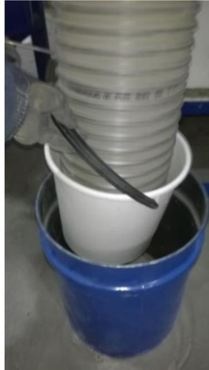
**Figure 41 Sampling from screen underflow**
