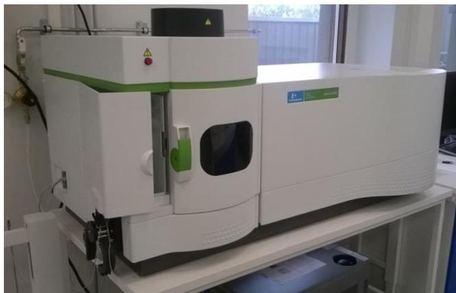
**Figure 19 ICP-OES used for element analysis**
