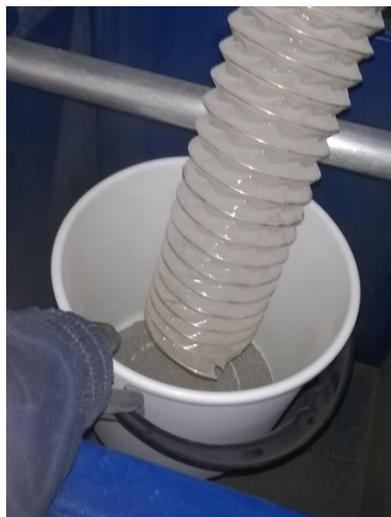
**Figure 39** Sampling for element analysis
