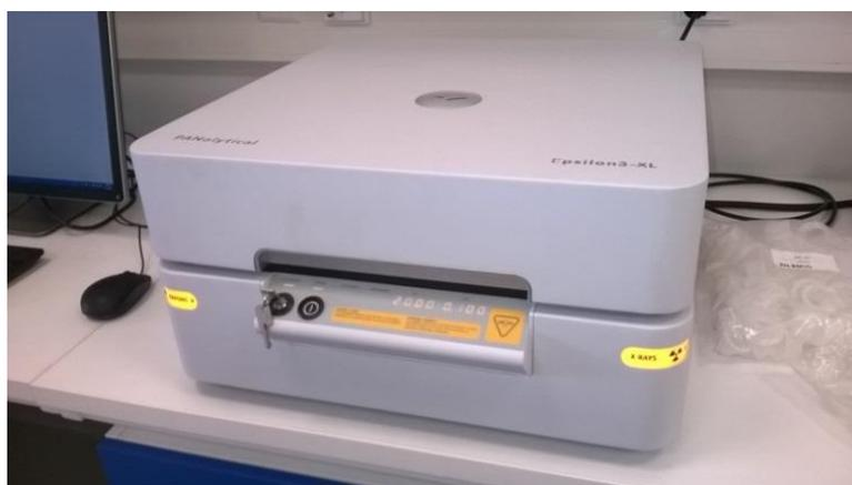
**Figure 17 XRF spectrometer used for element analysis**
