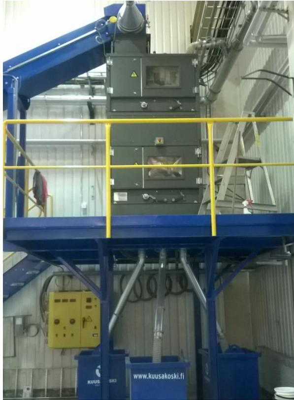
**Figure 15 Electrostatic separator used in the experiments**
