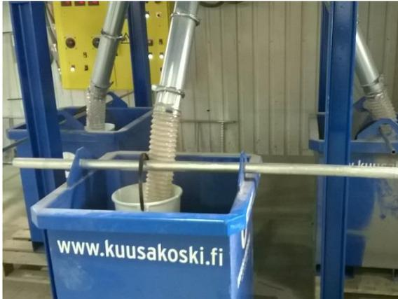
**Figure 37** Sampling for determination of mass fractions
