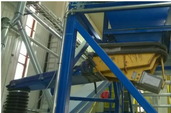
**Figure 11 Vibratory feeder**
