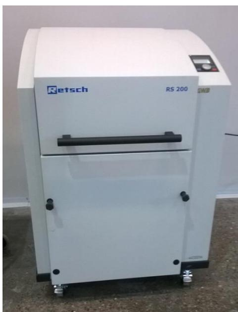
**Figure 18** Disc mill used for grind the samples
