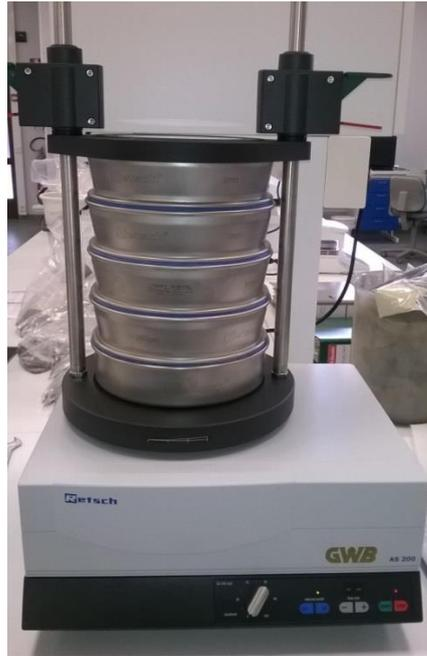
**Figure 21 AS200 Analytical Sieve Shaker by Retsch**
