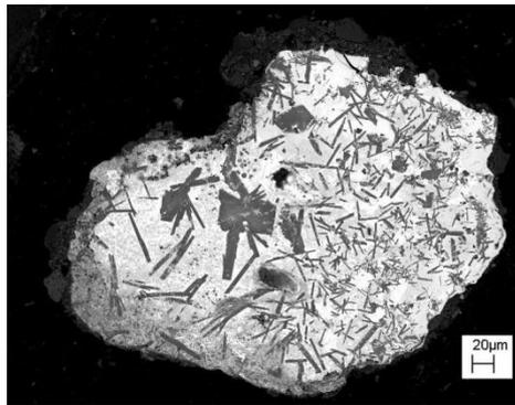
**Figure 31 F5. Particle with lead and oxides (aluminium, calcium, silicon). 10-20  $\mu\text{m}$  thick oxide layer on surface**
