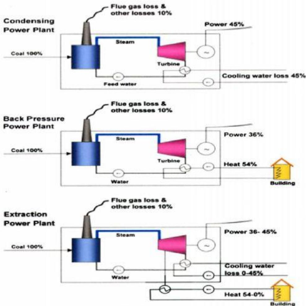
Figure 13. Condensing power plant with and without CHP technologies. (EURELECTRIC, 2014a)
