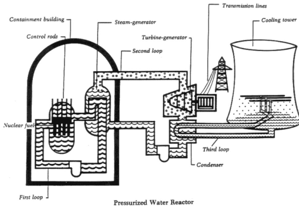
Figure 2. Pressurised water reactor. (NRC, 2012)
