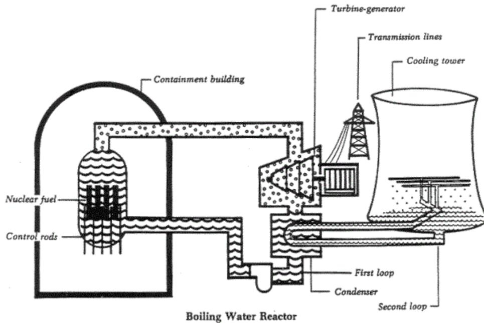
Figure 3. Boiling water reactor. (NRC, 2012)
