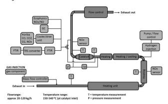
The exhaust gas temperature and flow can be independently adjusted with the research facility. The driving condition's selection was based on the emissions levels. In the selected driving mode, the engine out methane level was near 1000 ppm.
