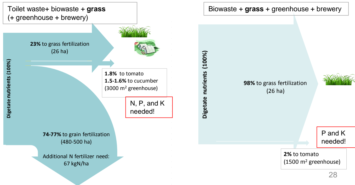
Figure 18: The nutrient flows in digestate utilization with and without toilet waste collection
