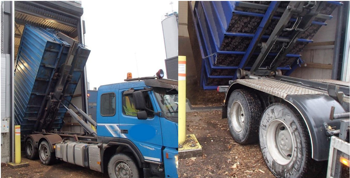
Figure 2. Rear-tipping of forest chips in a fuel receiving station of a power plant.
