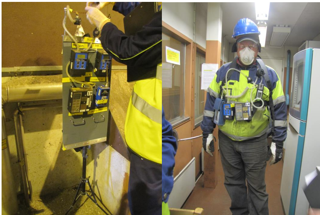
Figure 11. Stationary site sampling above 1.5 meter ground level during unloading (on the left) and truck drivers' exposure measurement from his breathing zone during unloading process of peat (on the right).
