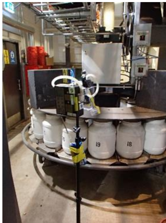
Figure 61. Automated fuel sampling system at a power plant.
