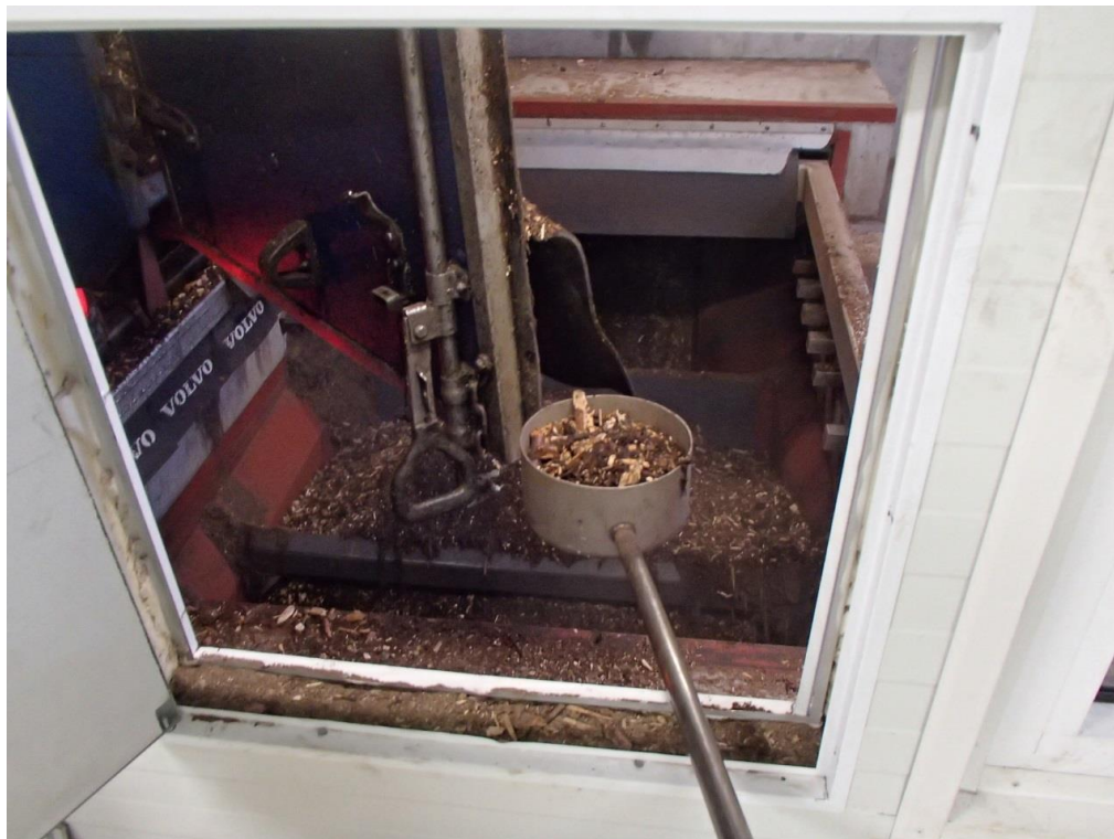
Figure 6. Sampling of fuel through a small window during unloading process.
