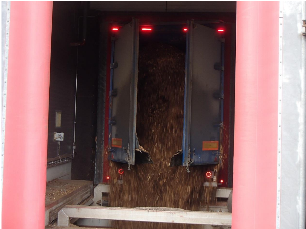
Figure 3. Rear-unloading of forest chips in a fuel receiving station of a power plant.
