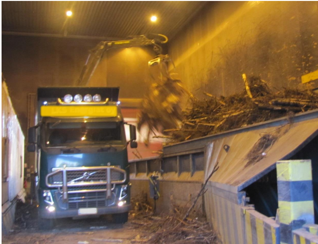
Figure 4. Unloading of forest residues for the crushing. The driver is sitting in a tight cabin equipped with air-conditioning system during the unloading.
