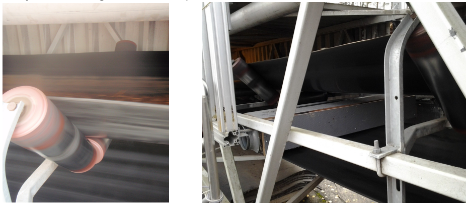
Picture 2. Left: Belt conveyor. Right: Detector's housing box between belts
