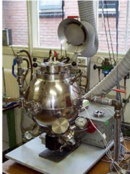
Figure 5. A 20-L sphere used for dust explosion measurements (Wilén et al. 2013). Photo: TNO.
