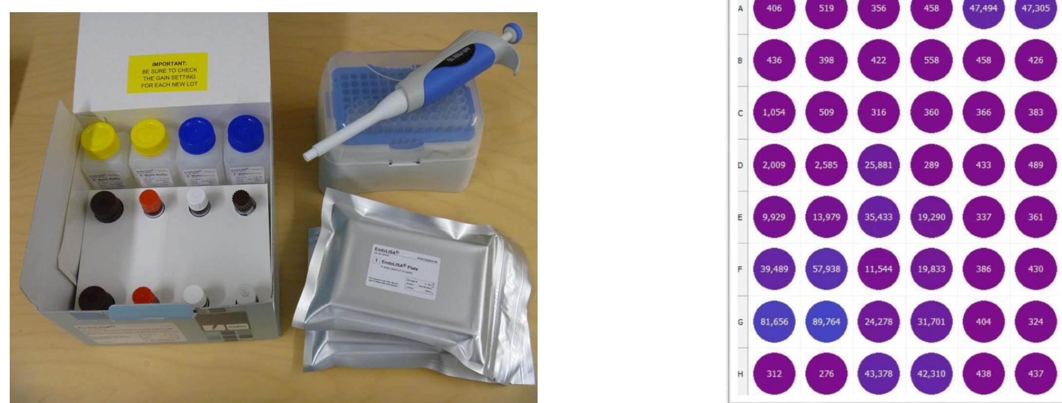
Figure 2. Left: ELISA-based assay for detection of endotoxins. Right: Results of the ELISA assay.
