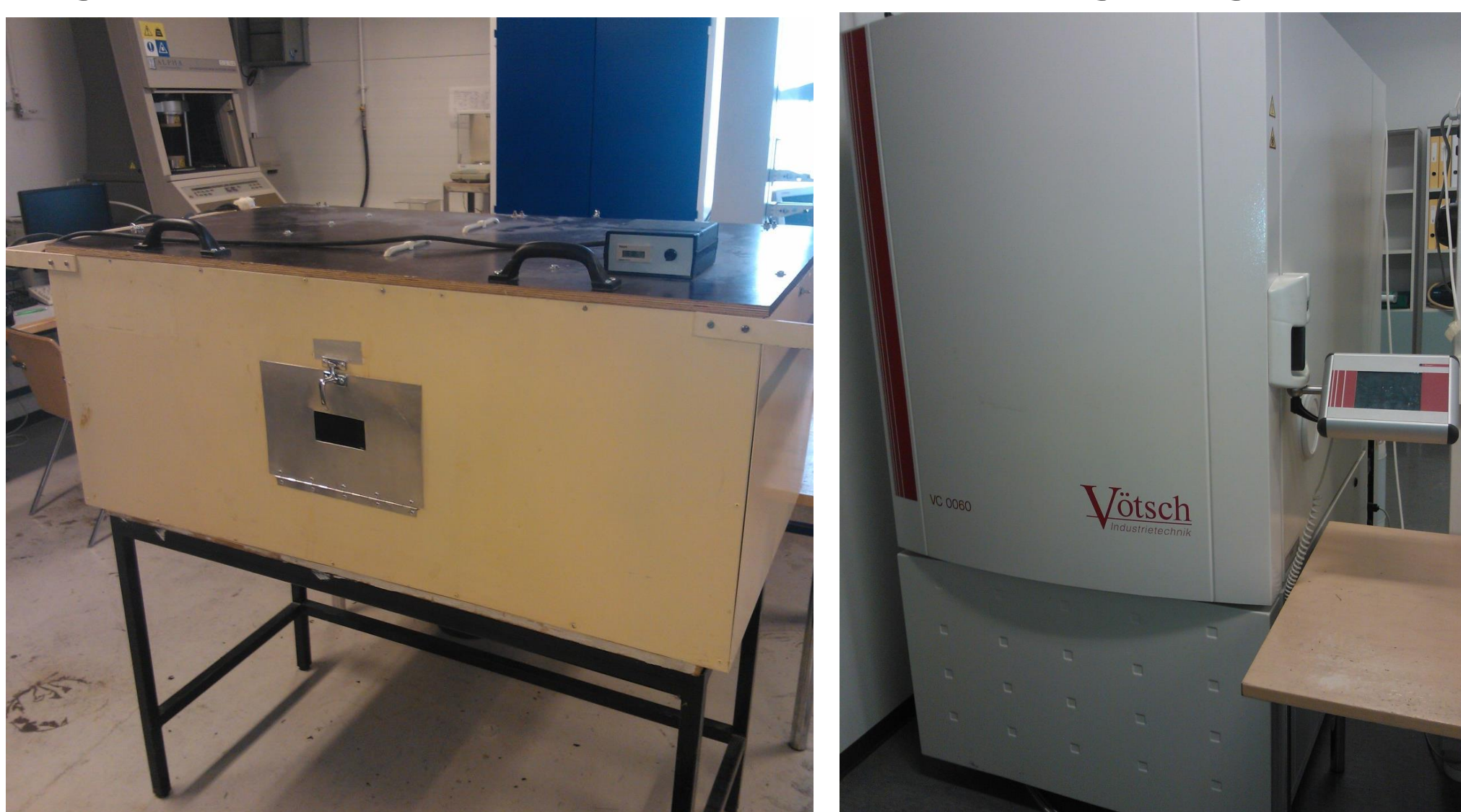
Fig.2. TUT's self built UV chamber and Vötsch climate testing equipment
