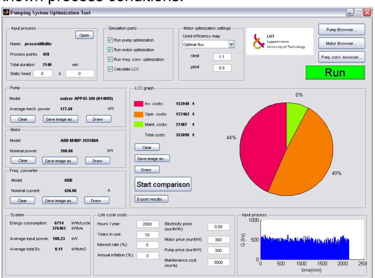
PSOT also allow easy comparison of existing and new pumping system for energy auditing purposes:
