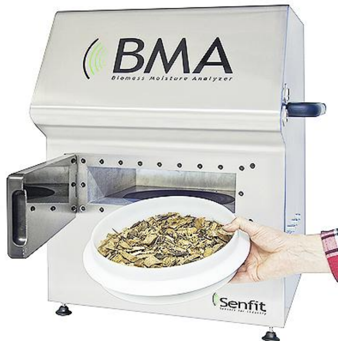
Image 8. Senfit BMA desktop moisture analyser based on microwave technology. (Image source [88].)
