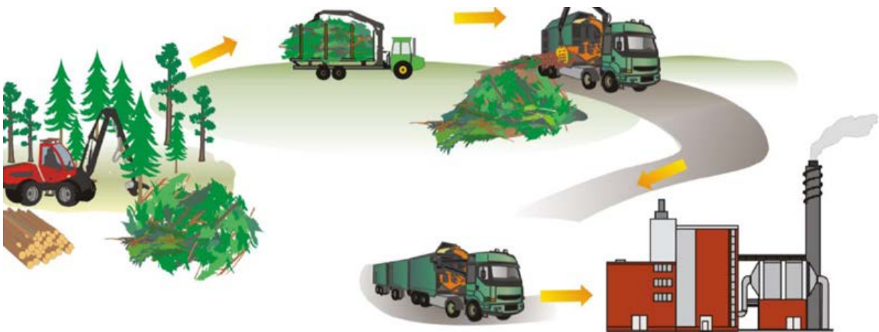
Image 1. The supply chain for logging residues where chipping is done at the roadside storage. (Image source [3])
