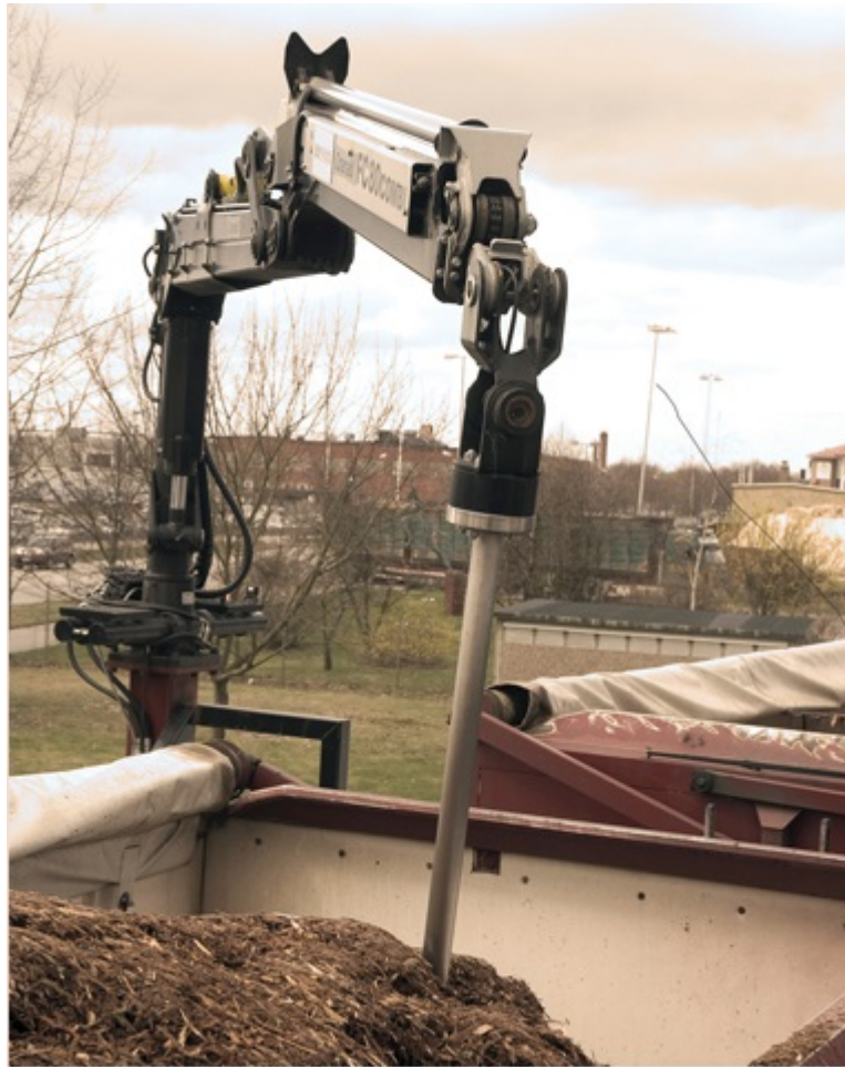
Image 17. Bestwood BAS-700A, a crane-based NIR-probe measuring moisture of a truck load. (Image source: [29])
