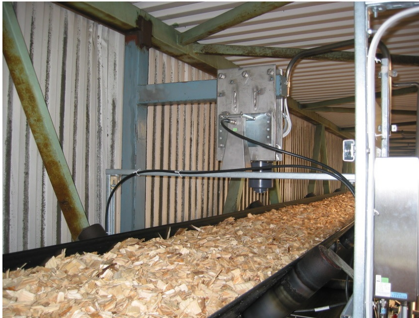
Image 14. Berthold LB 567/568 Micropolar microwave technology-based instrument measuring chip wood moisture online above the conveyor belt. (Image source [12].)
