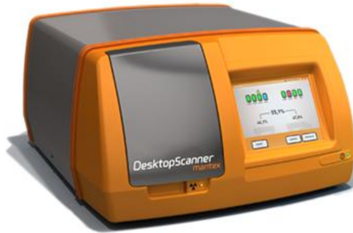
Image 10. The X-ray technology-based laboratory instrument Mantex Desktop Scanner. (Image source: [62].)
