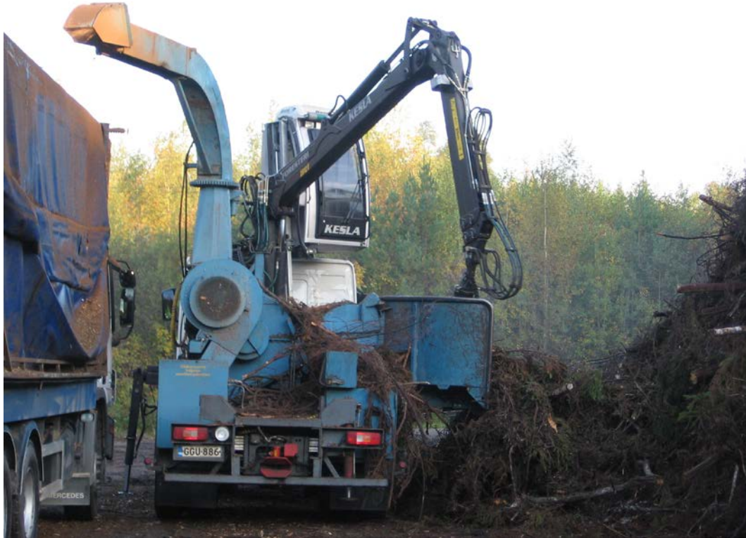
Image 4. Chipping the logging residues at the roadside storage. (Image Source: Jari Lindblad, Metla)
