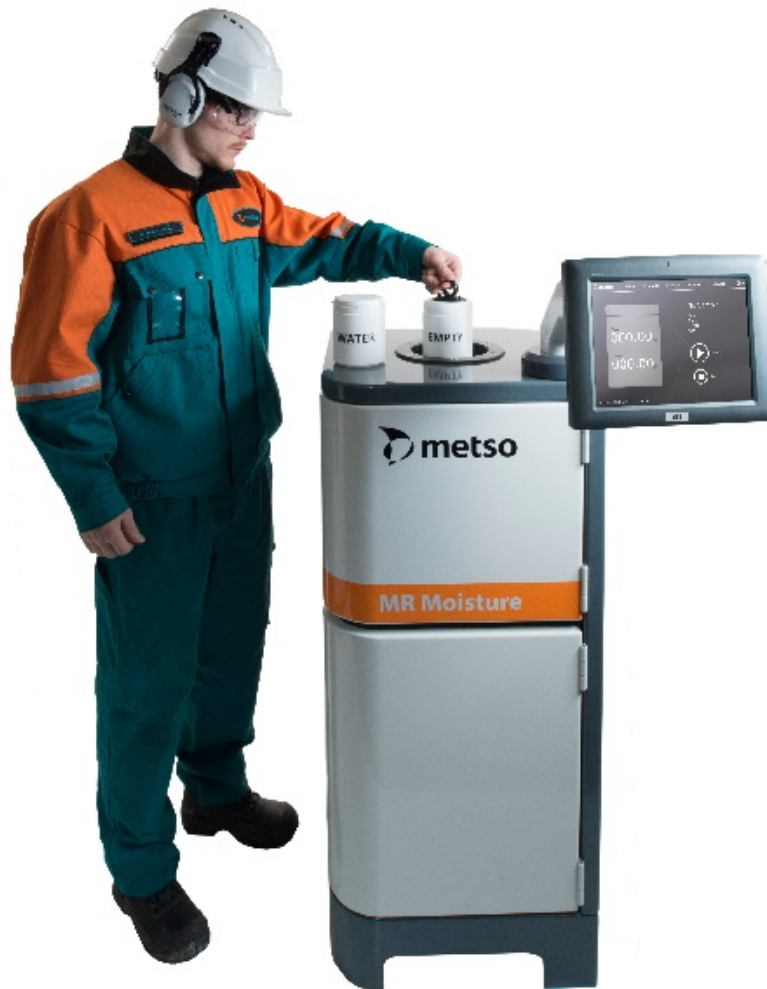
Image 9. Calibration of Metso MR bulk material moisture measurement instrument.
