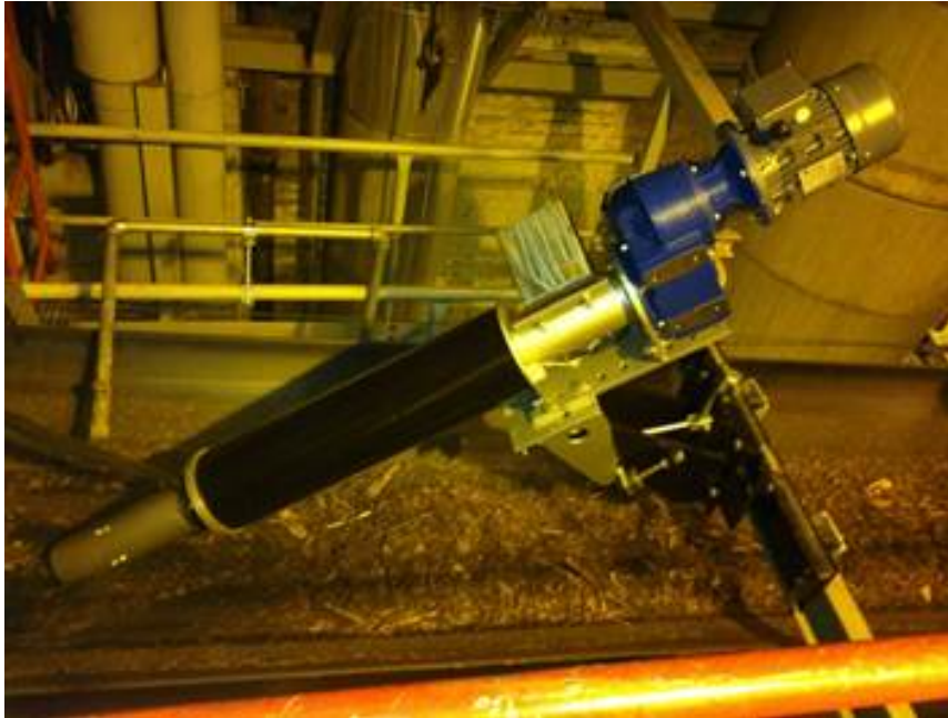
Image 12. Senfit BMA Online measuring moisture content of wood-based biomass on the conveyor belt. (Image source [88].)
