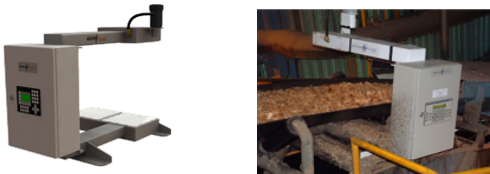
Image 13. Left: Moistscan MA500HD, the moisture measurement instrument based on microwave technology. Right: The instrument measuring wood chips in a pulp mill.
