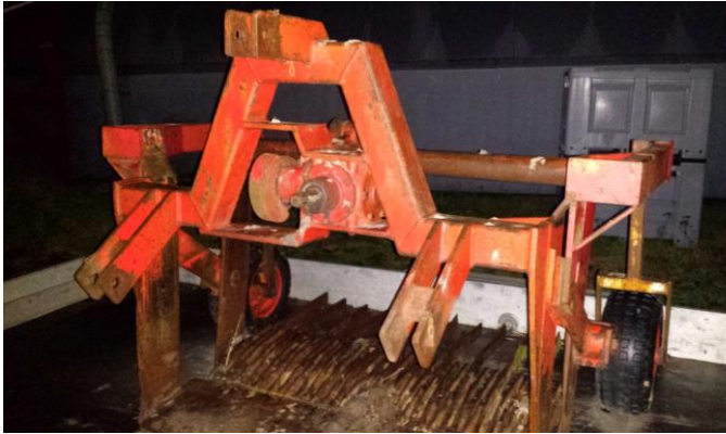
Seedlings lifting machine that shakes the soil off the roots
