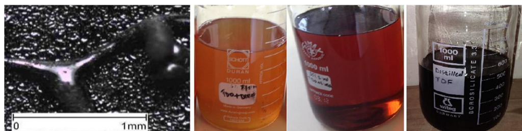
Crude, and distilled (< 150, 200, 250°C) rubber oils
