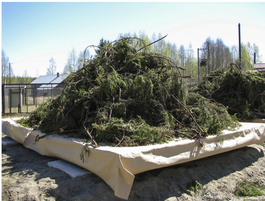
Fig. 3. Special drying platforms for simulating drying in a small logging residue pile in stand conditions.
