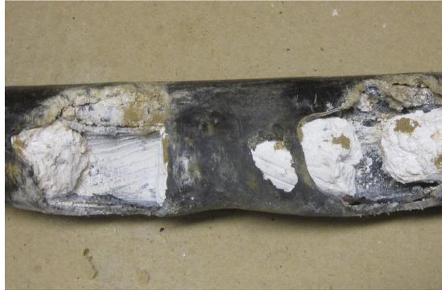
Figure 3.4. Permanently faulted part of an underground AXMK cable. Root cause of failure is probably a mole damaging the sheath.
