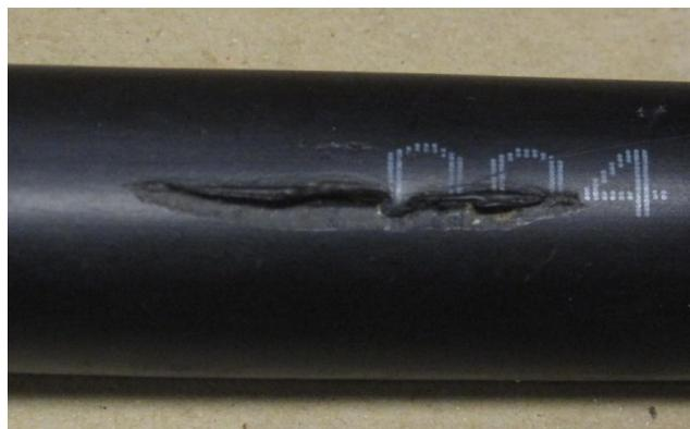
Figure 3.3. Cut in a sheath of an underwater AXMK cable. Probably caused by a propeller of an outboard engine.
