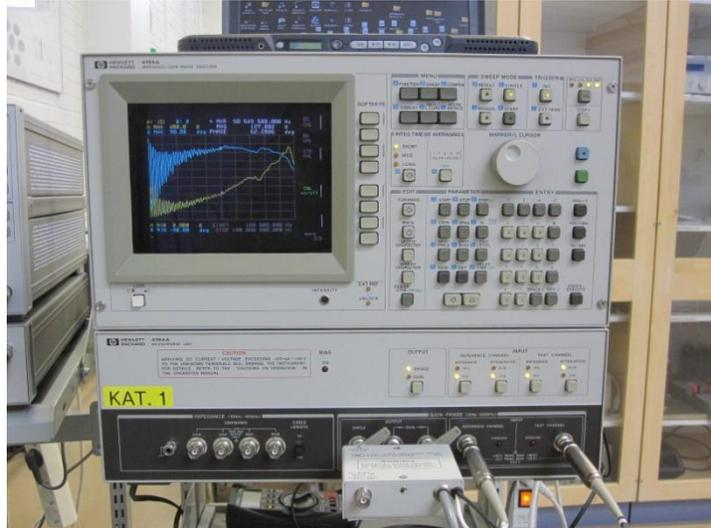
Figure 5.1. Hewlett-Packard 4194A impedance / gain-phase analyzer.
