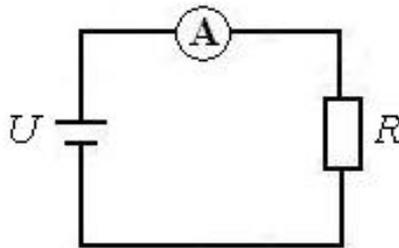
Figure 4.1. Basic concept of insulation resistance measurement.
