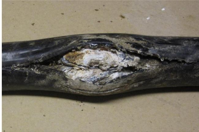
Figure 3.6. Permanently faulted double sheathed underground cable. Cable is probably damaged during the installation by ploughing.
