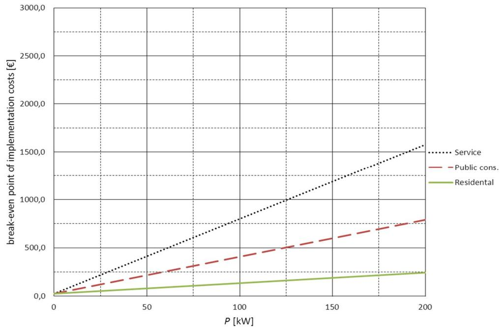
Figure 6.2. Break-even point of implementation costs of OCM to a single LV network as a function of average interruption power for different customer types. Interconnected network, no interruption when OCM is utilized and 2 h interruption without OCM.
