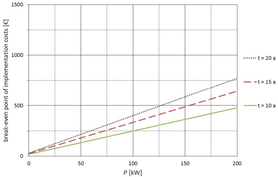
Figure 6.5. Break-even point of implementation costs of OCM to a single LV network as a function of average interruption power with different OCM system lifetimes. Interconnected network, no interruption when OCM is utilized and 2 h interruption without OCM. Average power is divided between 70 % residential type and 30 % service type customers.
