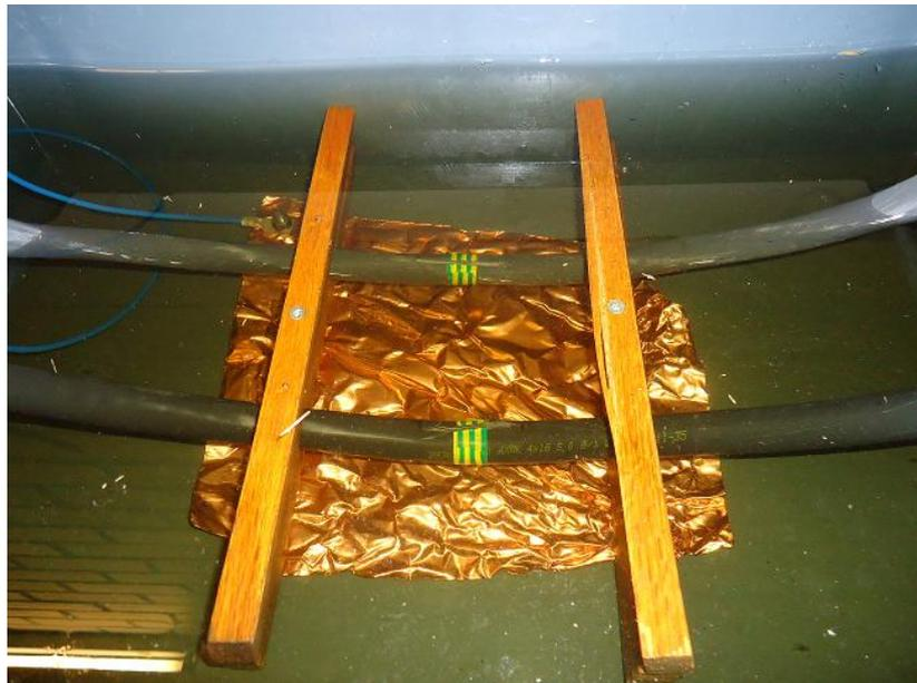
Figure 5.8. Submerged parts of first 50 m samples of both cable types with 5 cm long cut on the sheaths.
