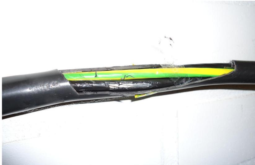
Figure 5.10. Final degree damage on brown phase insulation in AXMK cable.
