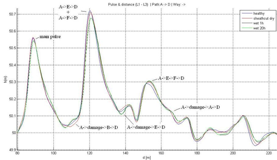
Figure 5.21. Results from gain & phase measurements from the grid point A to the point D presented in distance domain. Measured between L1 and L3 with the end of the branches being open. A value of  $0,72 \cdot c$  was used for signal propagation speed (Hernandez, 2012).
