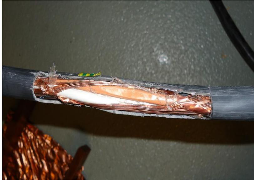
Figure 5.9. First degree damage on brown phase insulation in AMCMK cable.
