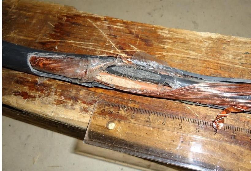
Figure 5.13. AMCMK cable with first degree damage done on brown and black phases.
