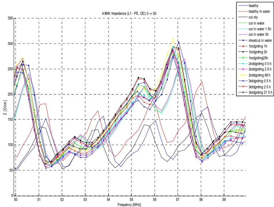
Figure 5.12. Impedance measurement results of progressive damaging of 50 m long AXMK cable sample. Close up view of Figure 5.11 of frequency band from 50 MHz to 60 MHz. Open circuit, measured between L1 and PEN.
