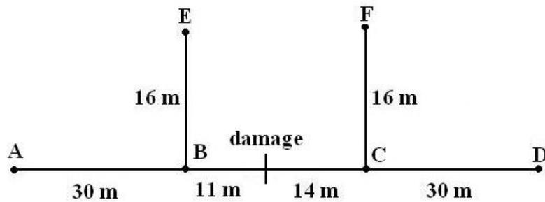
Figure 5.17. Topology of the grid setup. Grid consists of three segments of main line and two branches. Middle main line segment is damaged by cutting of a piece of sheath and submerging the cable under tap water.
