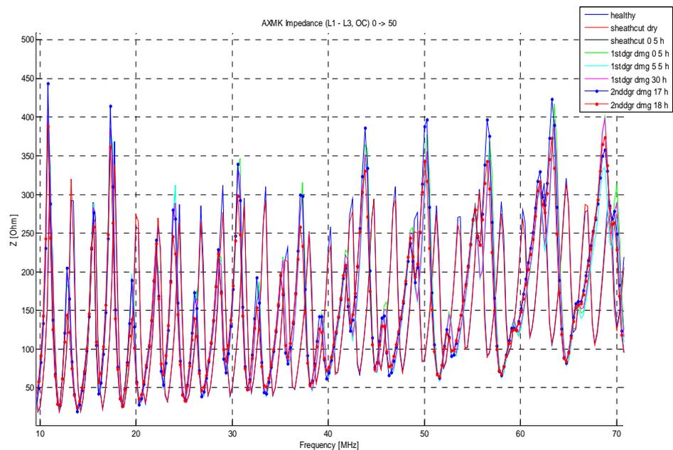
Figure 5.15. Impedance measurements of 50 m long AXMK cable sample with insulation around phases one and three gradually damaged in two steps. Open circuit, measured between L1 and L3.
