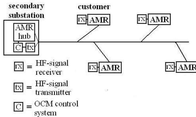
Figure 5.24. OCM system implemented to LV network with centralized read AMR meters.
