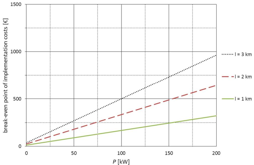
Figure 6.4. Break-even point of implementation costs of OCM to a single LV network as a function of average interruption power with different network lengths. Inter-connected network, no interruption when OCM is utilized and 2 h interruption without OCM. Average power is divided between 70 % residential type and 30 % service type customers.
