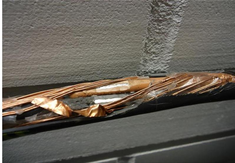
Figure 5.14. AMCMK cable with second degree damage done on brown and black phases.
