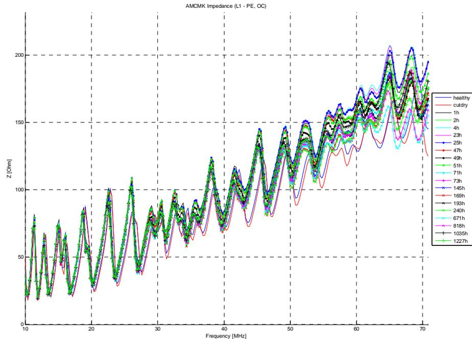
Figure 5.6. Long term impedance measurements of 25 m AMCMK cable sample. Number of hours on different curves point out the duration of which cable has been submerged under tap water with section of sheath removed. 'Healthy' and 'cutdry' are measured in dry conditions. Open circuit, measured between L1 and PEN.
