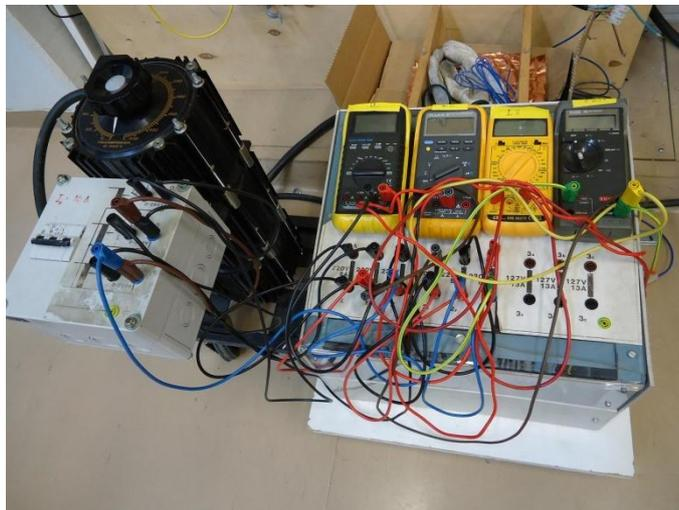
Figure 5.2. Voltage test setup. Variable autotransformer is connected to 1:1 isolation transformer in order to achieve galvanic isolation of damaged cables from common ground potential. Transformer neutral is connected to a copper plate located in water tank to provide a return path to possible phase – to – ground leakage current from damaged non-concentric AXMK cable. Phase currents and returning current from copper plate were measured using regular multimeters.
