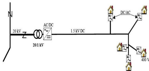
Figure 2.5. A basic concept of LVDC distribution. (Kaipia et al. 2006)
