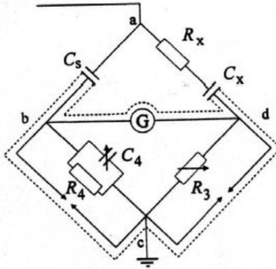
Figure 4.3. The Schering bridge (Aro et al. 2003).
