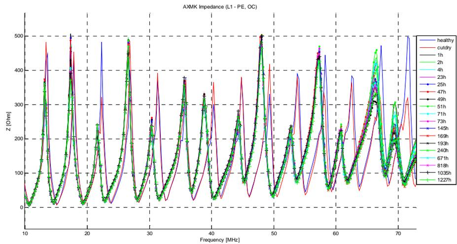
Figure 5.5. Long term impedance measurements of 25 m long AXMK cable sample. Number of hours on different curves point out the duration of which cable has been submerged under tap water with section of sheath removed. 'Healthy' and 'cutdry' are measured in dry conditions. Open circuit, measured between L1 and PEN.
