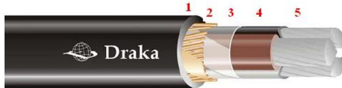
Figure 2.2. Concentric AMCMK 1 kV cable, where 1) is outer protective sheath, 2) concentric conductor, 3) polypropene bands, 4) phase insulation, 5) aluminum conductors. (Modified from Draka, 2011).
