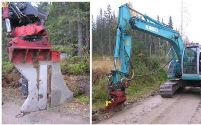
Figure 3.1. a) Cable plough b) Ploughing of AMCMK-PE -cable (Reka 2011)
