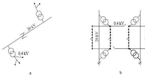
Figure 2.1. Typical a) rural and b) urban LV network. The black dots represent customers connected to the network. (Lakervi & Partanen, 2009).
