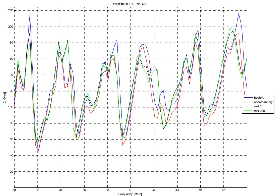
Figure 5.20. Impedance measurement results of grid setup from the point A. Open circuit, measured between L1 to PEN. Close up view of Figure 5.19 of frequency band from 30 MHz to 50 MHz.
