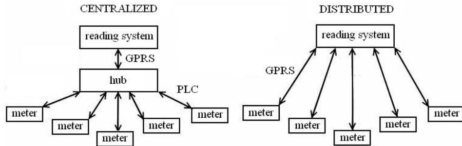
Figure 5.23. Examples of centralized and distributed communications between AMR reading system and meters. (Modified from: Valtonen, 2009)
