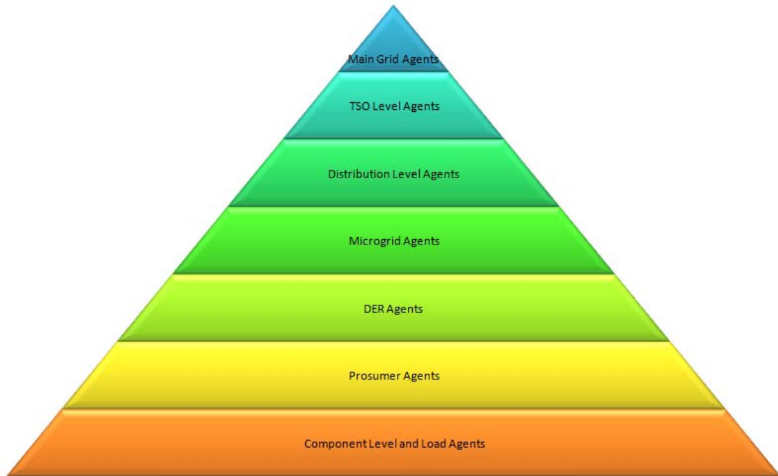
Figure 6.1 Seven Layers Control Architecture of Micro Grid
