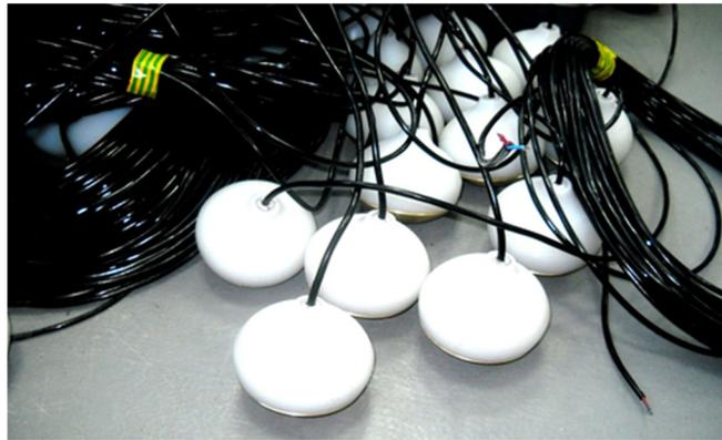
Figure 50. Shallow water bottom geophone units built within the scope of CCSP
