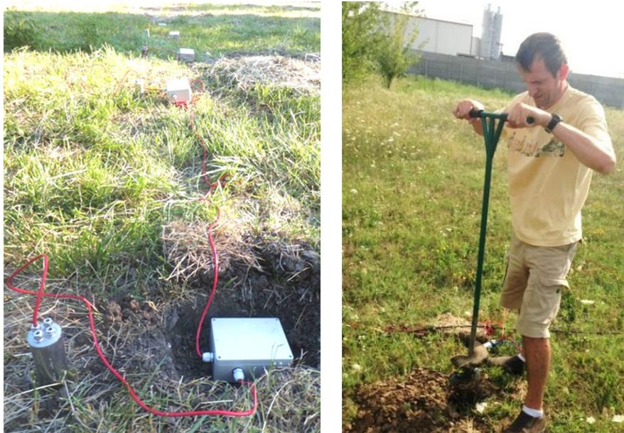
Figure 52. Testing the subsurface permanent seismic array. The steel cylinders house 3-component geophones and/or a vertical low frequency geophone. They are to be installed at approximately 2m depth by means of an auger drill (right). The grey boxes contain the acquisition and transmission electronics and are to be buried at 0.5-1m depth (left), hiding the system from activities carried on the surface above.
