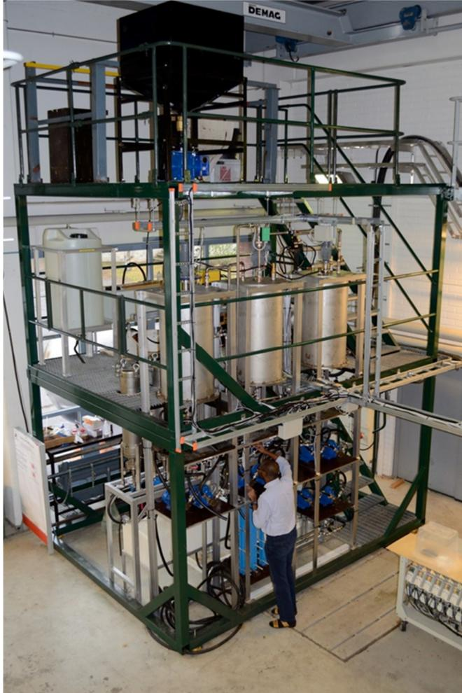
Figure 62. Completed Slag2PCC pilot plant (photo by S.Teir).
