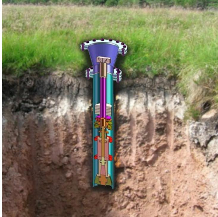
Figure 54. Design of the subsurface seismic source. A low power multi-impact device produces vertical pulses. The bottom of the borehole is prepared to maximise the energy transfer from the mechanism to the ground.
