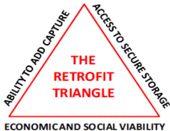
Figure 5. The "Retrofit triangle" shows the three separate, though interlinked, requirements that need to be satisfied in order to a retrofit project to be viable. (Gibbins, et al., 2011)
