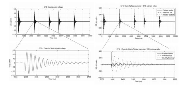
**Figure 3.** Neutral point voltage and sum of phase currents and close-ups in 10 seconds time interval. (Dlaboratory Sweden Ab. 2012.)
