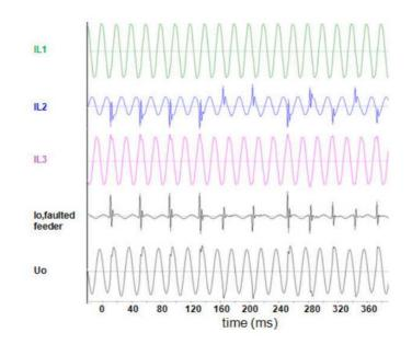
**Figure 5.** Phase currents, zero sequence current at the faulted feeder and neutral point displacement voltage from a real situation, which led to substation disconnection. (Wahlroos 2012.)
