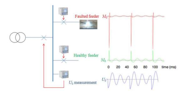
**Figure 1.** Residual currents of faulted and healthy feeders and neutral point displacement voltage waveform in intermittent earth fault situation. (Wahlroos 2012.)
