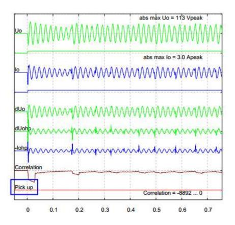
Figure 12. Field test data of healthy feeder. (Kumpulainen 2008.)
