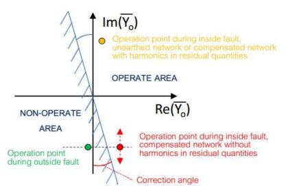
**Figure 13.** Operation characteristic for multi-frequency admittance protection method. (Wahlroos et al. 2013.)
