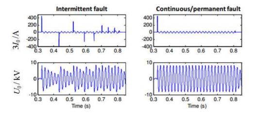
**Figure 7.** Comparison of intermittent erath fault waveforms and permanent earth fault waveforms. (Wahlroos et al. 2011.)
