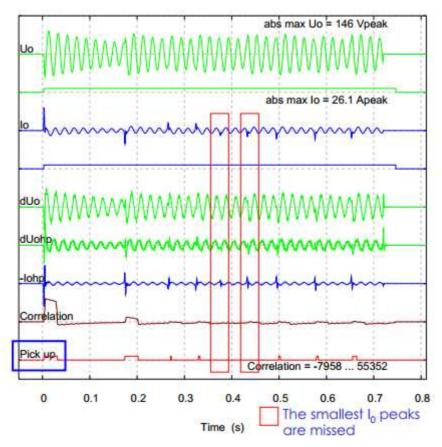
Figure 11. Field test data of faulty feeder. (Kumpulainen 2008.)
