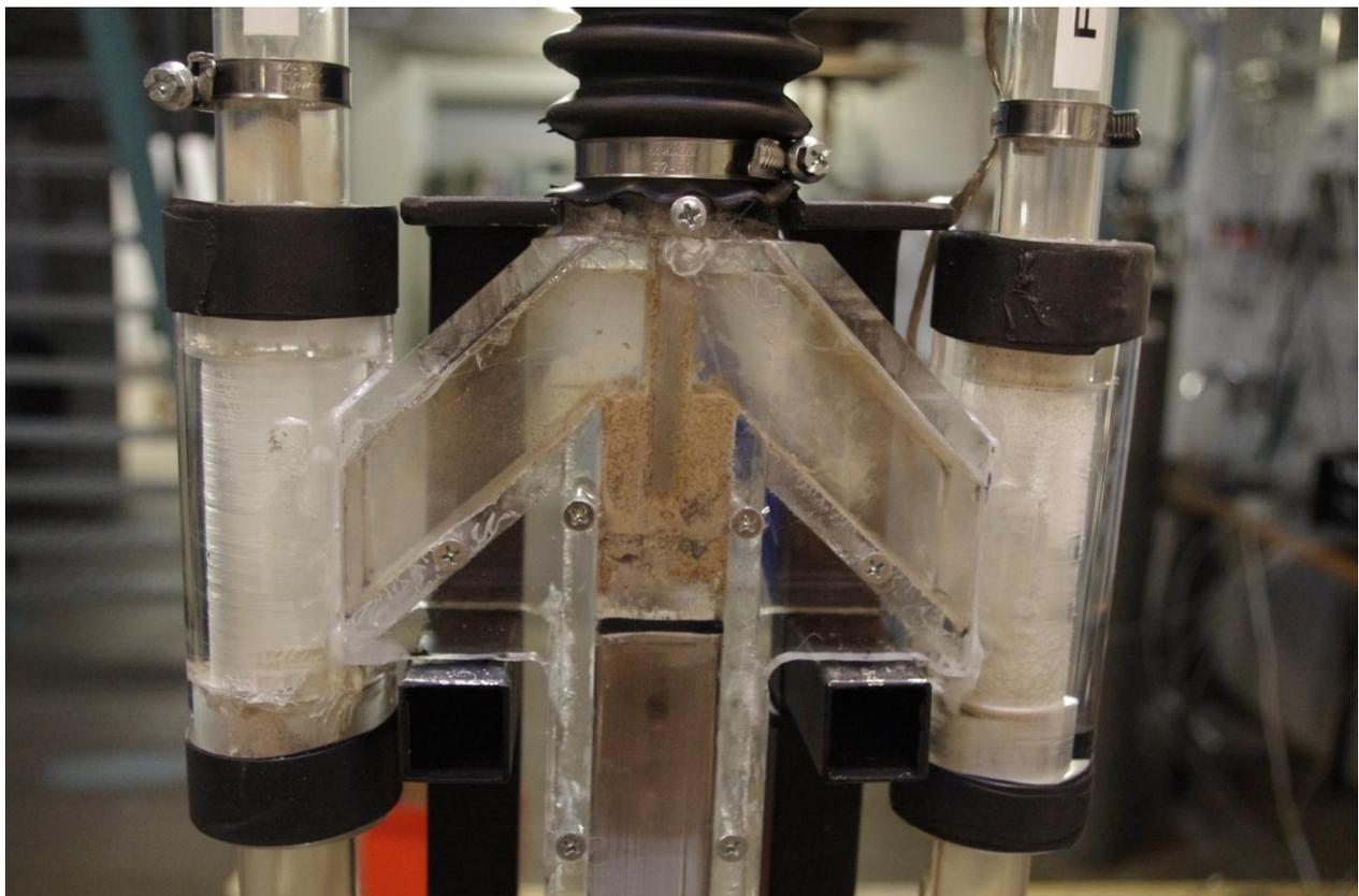
Figure 6. Double exit loop-seal; recycle chambers filled with sand
