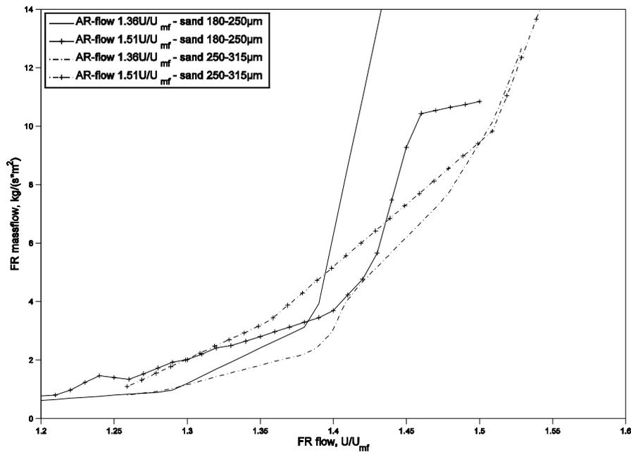
Figure 4. Solid mass flow to the FR-side with different particle size distribution.
