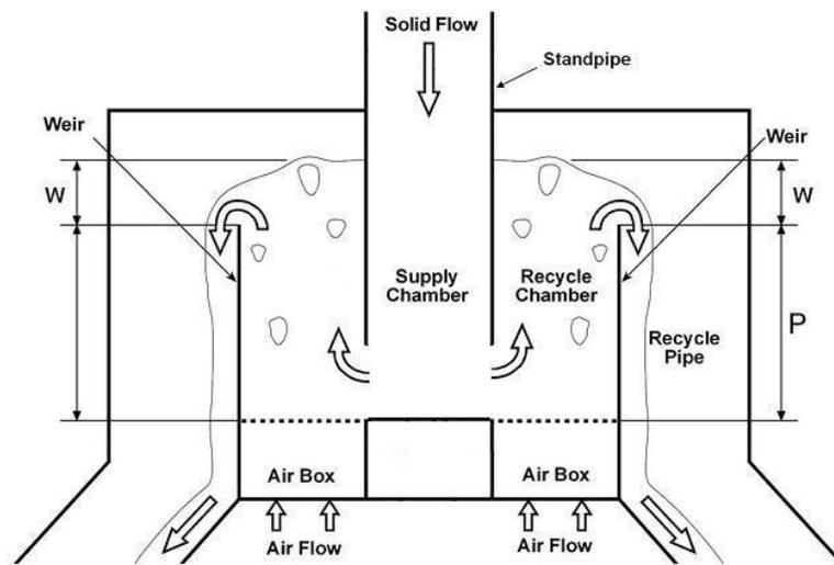
Figure 5. Schematics of the double exit loop-seal used at experiments.
