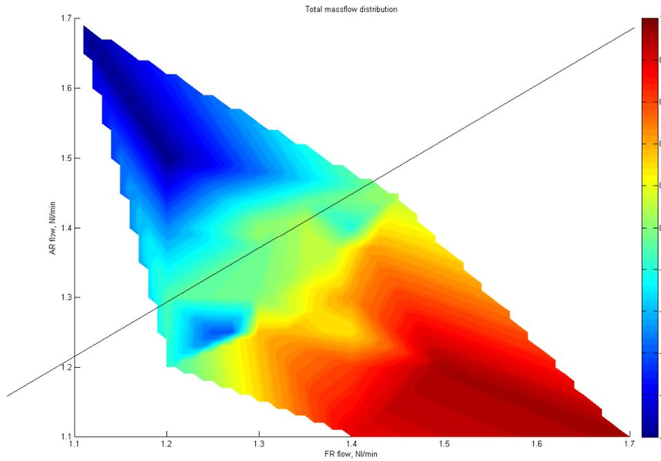
Figure 8. Fluidization velocity effect to mass flow distribution between recycle chambers, sand 180-250 $\mu$ m. 1 all solids to FR-side, -1 all solids to AR-side, 0 even distribution between recycle chambers. Line presents approximate 0-level where distribution is even. 0-level is shifted to AR-side because of leakage of fluidization air from FR-side.
