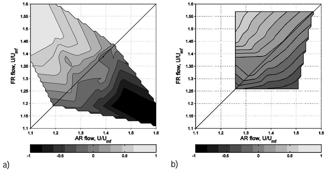
Figure 3. Fluidization velocity effect to mass flow distribution between recycle chambers, a) sand 180-250µm, b) sand 250-315µm. 1 all solids to FR-side, -1 all solids to AR-side, 0 even distribution between recycle chambers.
