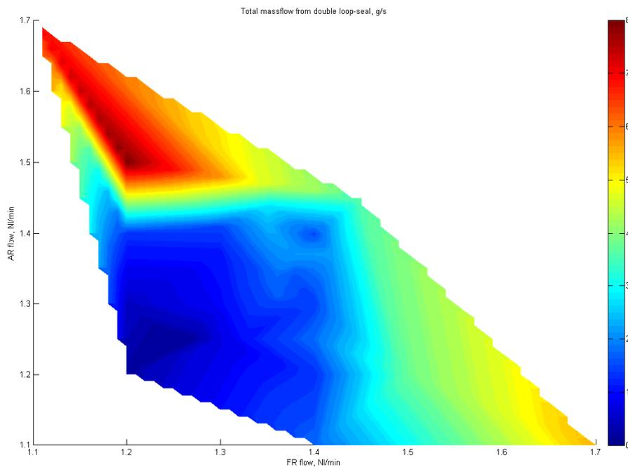
Figure 9. Fluidization velocity effect to mass flow over double loop-seal (g/s), sand 180-250 $\mu$ m. Blue area contains area where fluidization is stable and well controlled, below 1.4 NI/min  $\approx$  1.45 $U/U_{mf}$ .
