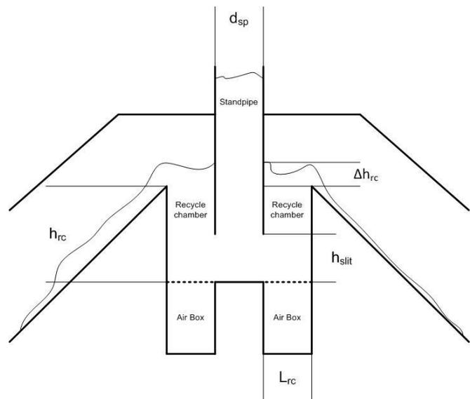
Figure 1b. Schematics of the double exit loop-seal used at experiments.
