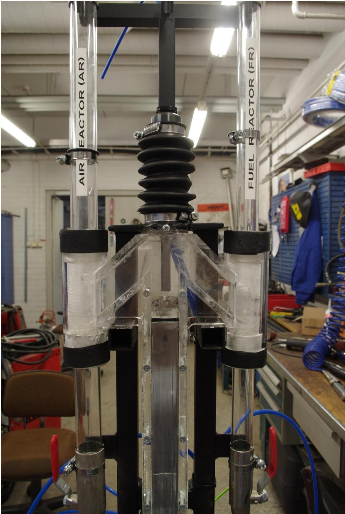
Figure 7. Double exit loop-seal after grate revision with reinforced structure
