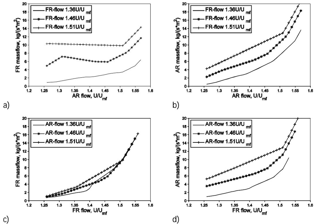
Figure 2. Effect of fluidization velocities to solid mass flow at different recycle chamber, sand 250-315 $\mu\text{m}$ . a) mass flow to the FR-side depending on fluidization flow to AR-side, b) mass flow to the AR-side depending on fluidization flow to AR-side, c) mass flow to the FR-side depending on fluidization flow to FR-side, d) mass flow to the AR-side depending on fluidization flow to FR-side.
