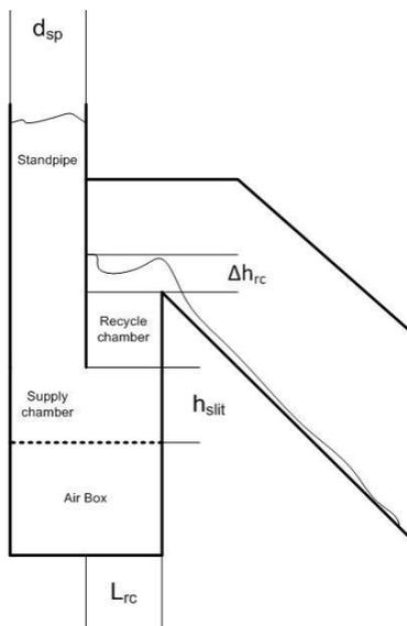
Figure 1a. Schematics of loop-seal
