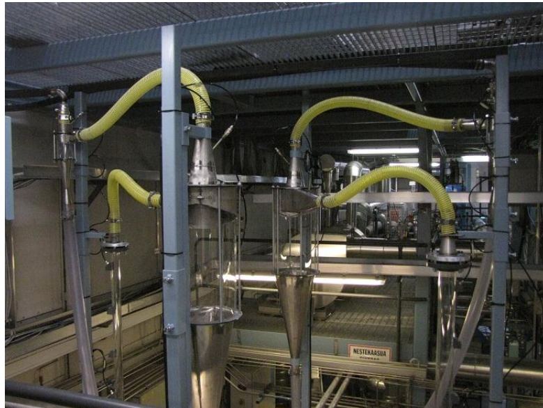
Fig. 7 Cyclones at the top of test rig. Primary cyclones are at the middle and secondary cyclones are on the edge of picture. Black tubes from secondary cyclones are connected to bag filter.
