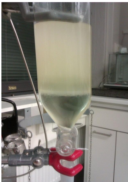
Figure 4. Settling of two liquid phases after CO 2 bubbling (Uusi-Kyyny 2014).
