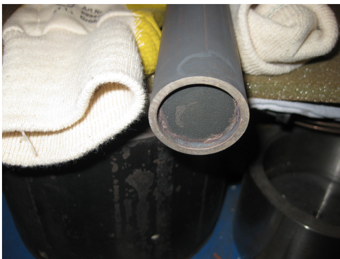
Figure 3. The sintered filters installed to fluidization tube cover and to fluidization tube bottom.
