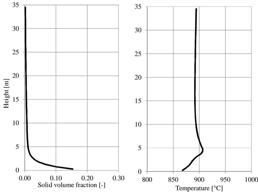
Figure 6. 1D solid volume fraction profile and temperature profile of the calciner.
