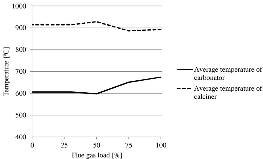
Figure 9. Average temperatures of the reactors in different loads. Several parameters affect the development temperatures in the reactors which in term have an effect on gas velocities. This creates a difficulty in controlling solid fluxes.
