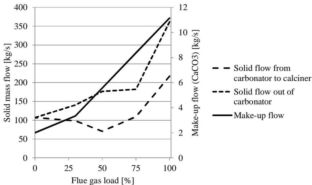
Figure 10. Solid flow out of the carbonator and solid allowed to the carbonator plotted as a function of flue gas load (left hand side axis). The solid mass flow has a lot of variation because it is dependent on several variables like gas velocity and reactor solid inventory and inventory composition.
