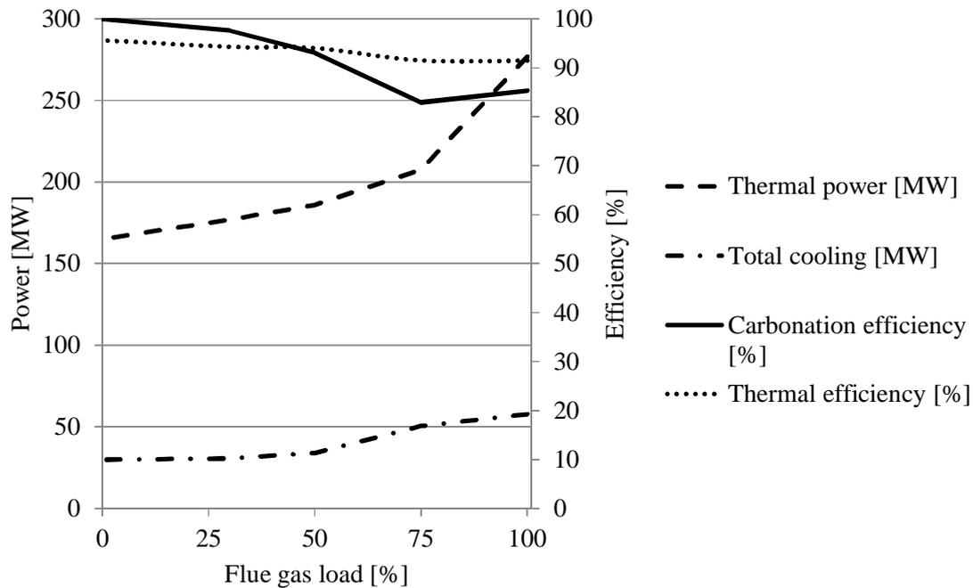
Figure 7. Thermal power of the calciner and total cooling of the carbonator plotted as a function of the flue gas load on the left hand side axis. In the same figure, carbonation efficiency and thermal efficiency of the calcium loop are plotted as a function of flue gas load (right hand axis).
