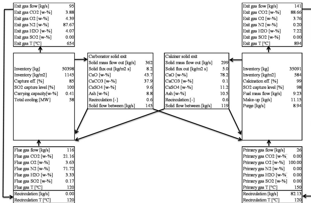
Figure 3. Overall balance of the full load calculation case.
