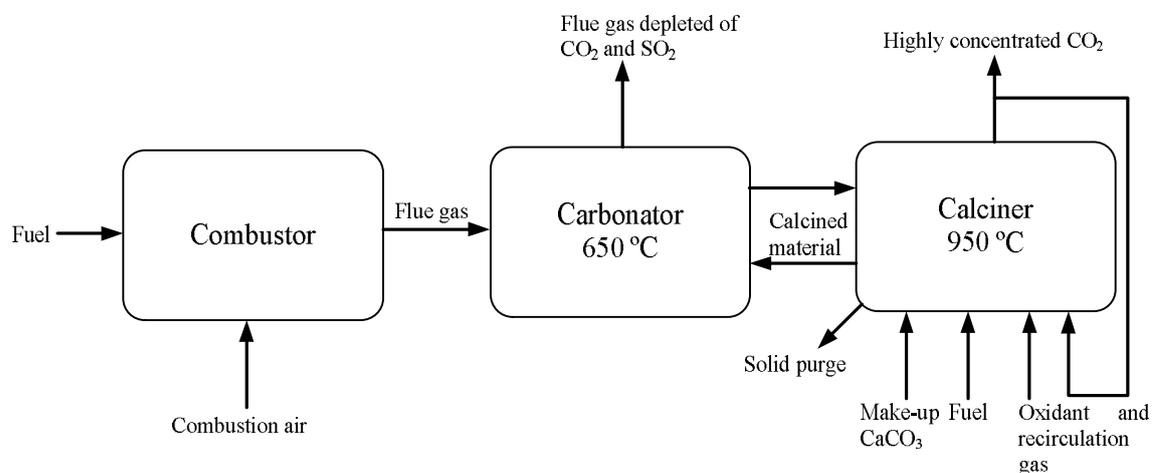
Figure 1. Concept of the calcium looping process.
