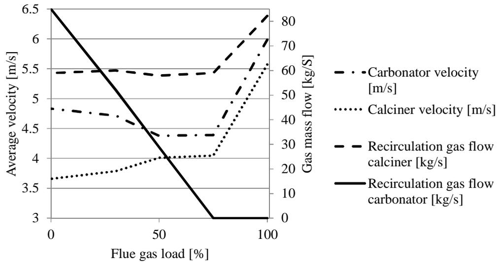
Figure 8. Recirculation gas flow to reactors in different load scenarios (right hand axis). Left hand axis presents the average velocity of the reactor in different load scenarios. Keeping average gas velocity close to the desired value becomes difficult in low flue gas loads.
