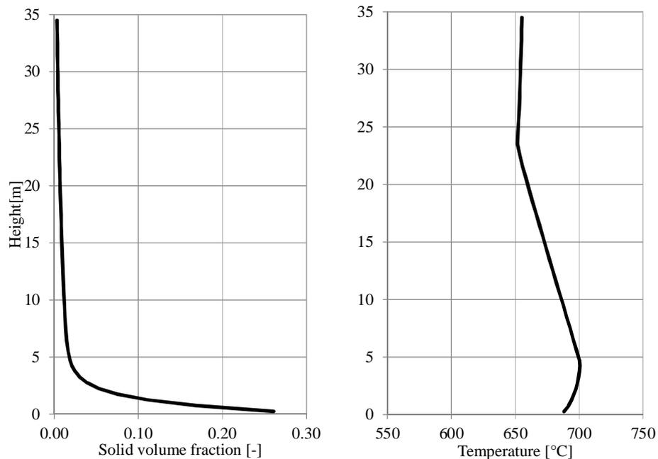
Figure 5. 1D solid volume fraction profile and temperature profile of the carbonator.
