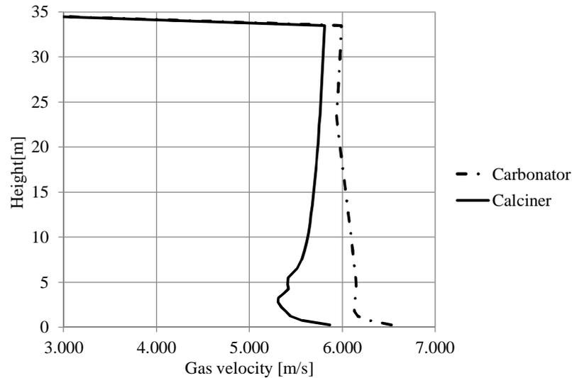
Figure 4. 1D velocity profiles of the reactors from full load calculation case.
