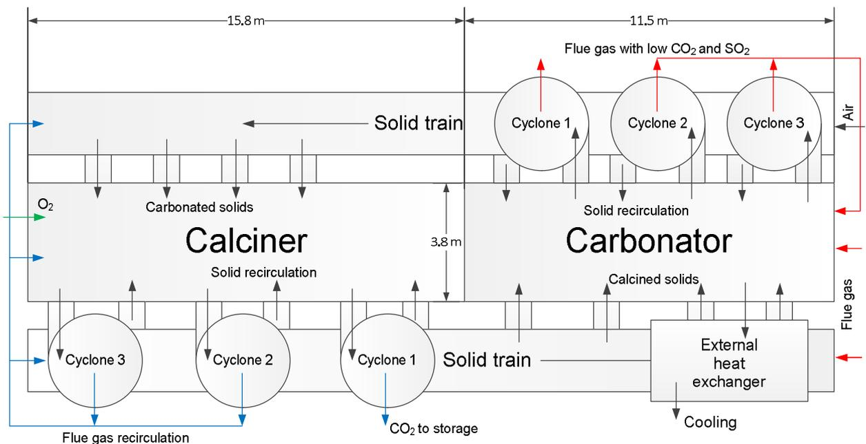
Figure 2. Simple dimensioning of the concept unit, with the external heat transfer block and solid/gas paths.
