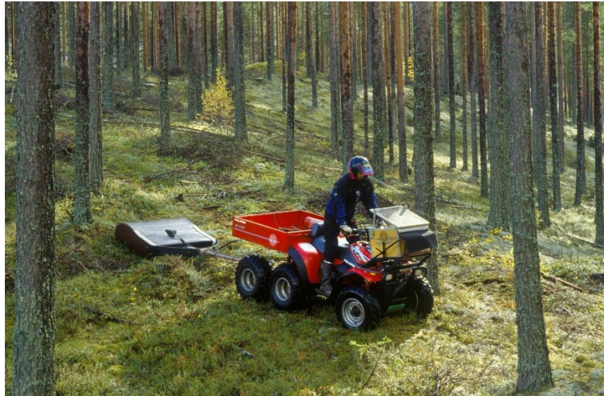
Figure 12. Ground penetrating radar. Photo Jari Väätäinen, Geological Survey of Finland.
