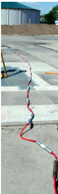
Figure 49. Receiver string used for cross-hole measurements and its installation in borehole KTZI-202.
