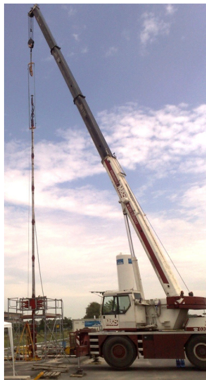
Figure 49. Receiver string used for cross-hole measurements and its installation in borehole KTZI-202.
