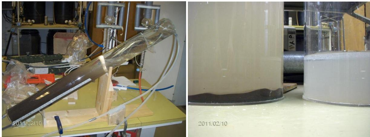
FIGURE 4.2 Inclined settler at 30° angle (right) and reactor samples from the experiment (left).
