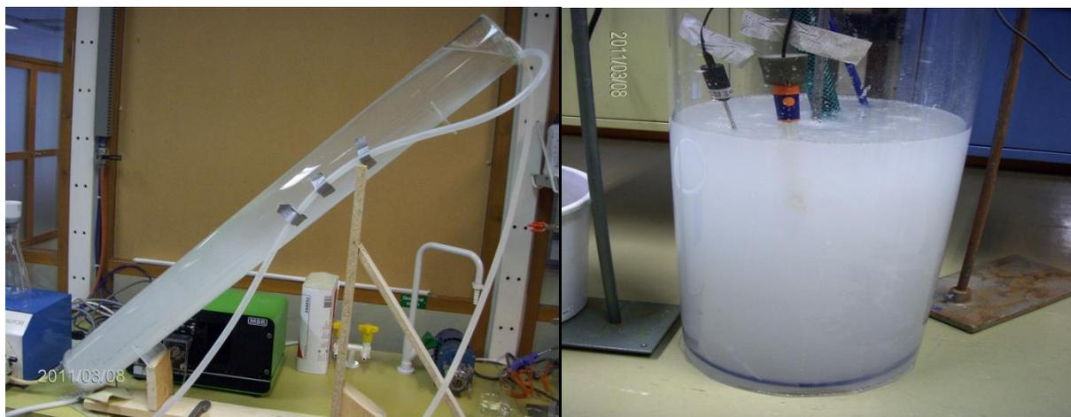
FIGURE 5.2 The separator (left) and reactor (right) in carbonation experiment.
