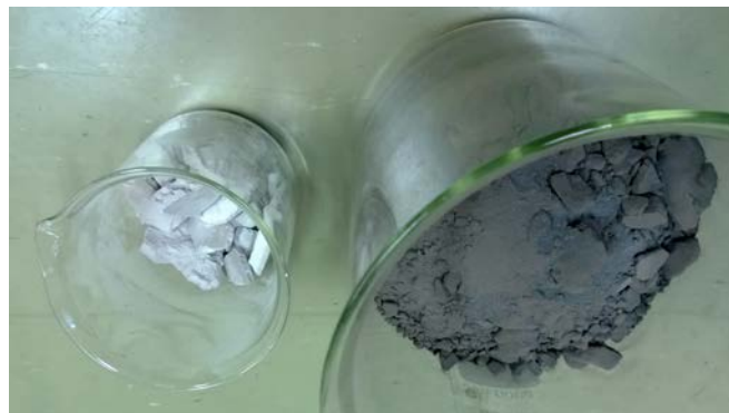
Figure 4. Produced PCC (left) and residual slag (right) from a continuous experiment run with the demo setup.
