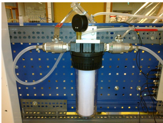
Figure 19 Filter element used after inclined settlers at ÅA
