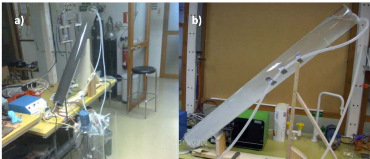
Figure 18 a) inclined settler for slag sedimentation; b) inclined settler for PCC sedimentation (Filppula, 2012)
