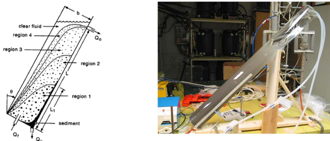
Fig. 7 Inclined settlers: concept (left) (Davis and Gecol, 1996) and tests with steelmaking slag at ÅA (right) (Filppula, 2012)
