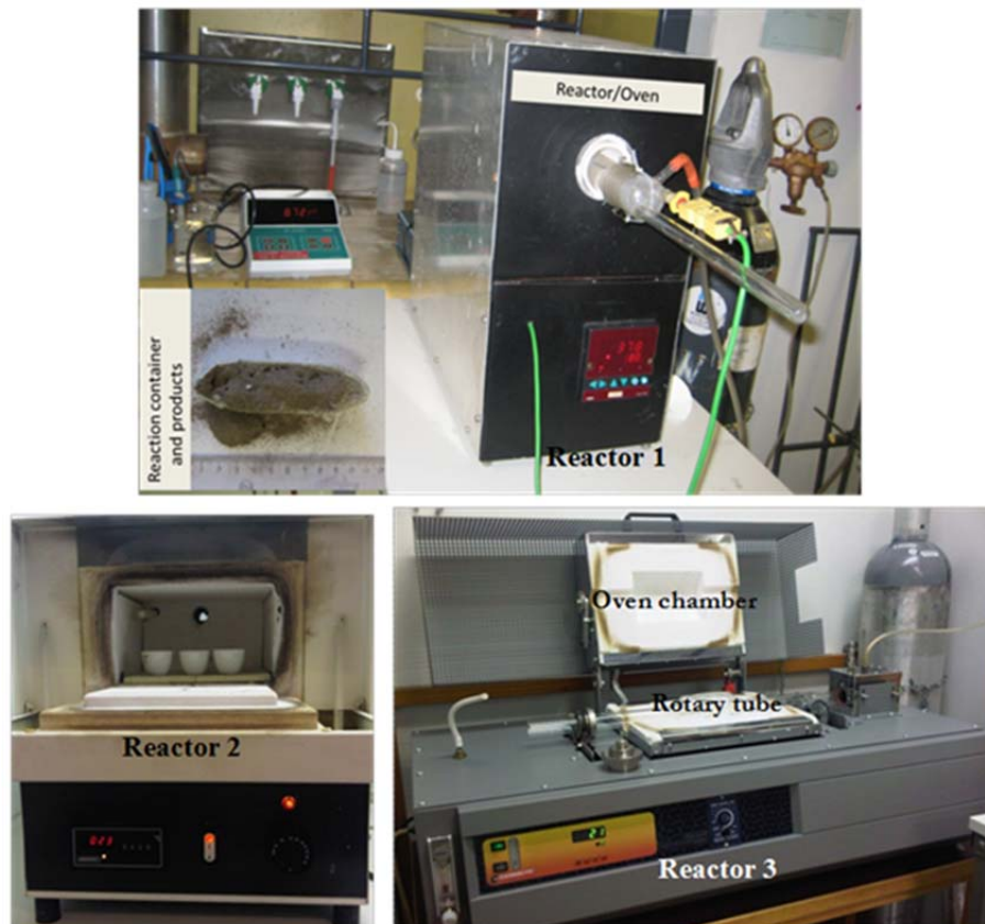
Fig. 2 Reactors used for solid/solid conversions at ÅA
