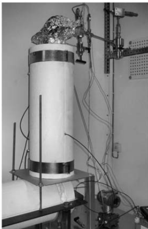
Fig. 4 Reactor used for carbonation conversion at ÅA
