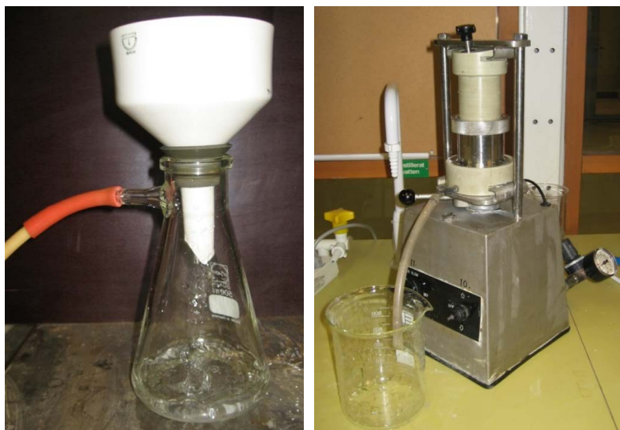
Figure 3.2.17 The vacuum filter (left) and the pressure filter (right) used for the experimental tests.
