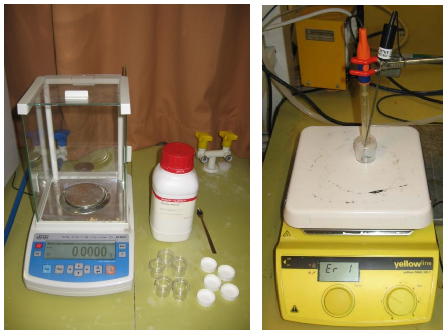
Figure 3.1.9 Scale, calcium carbonate, batches, pH- and temperature- meter and magnetic stirrer used for the experiment.
