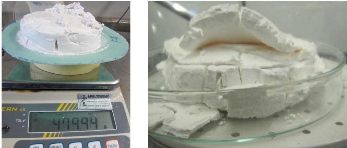
Figure 4. A typical filter cake from the experiments after pressure filtration on the left-hand side and a cake produced by S-PCC+ ammonium acetate after dry matter determination on the right-hand side.
