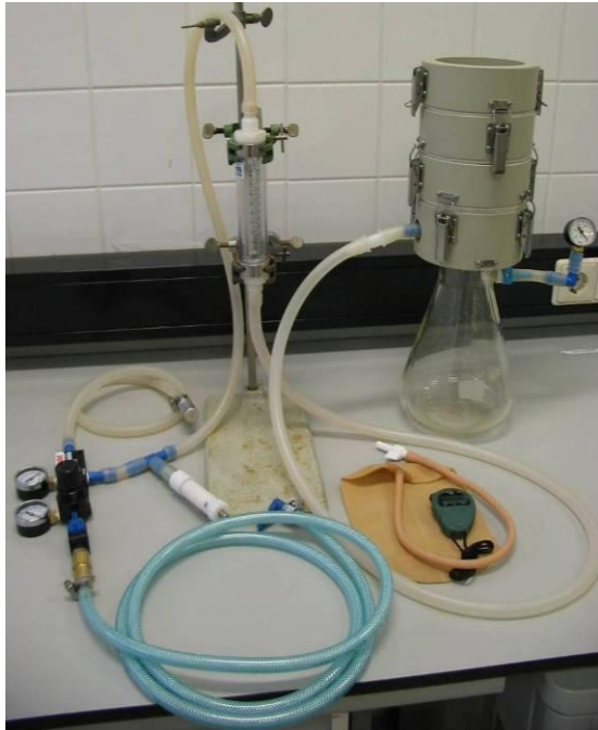
Picture 3. Outotec Larox® Büchner (BVB) test unit.
