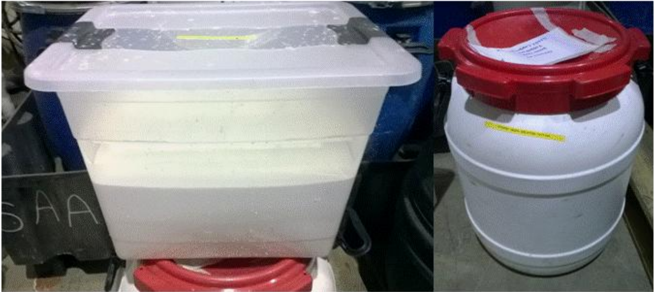
Picture 4. Container that had the slurry on the left, and container for the dilution liquid on the right.
