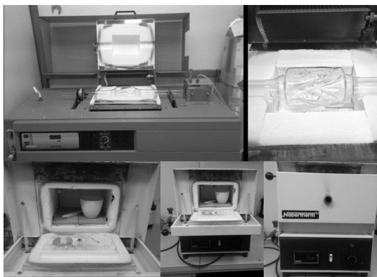
Figure 5. Rotary tube (above) and chamber furnace (below).
